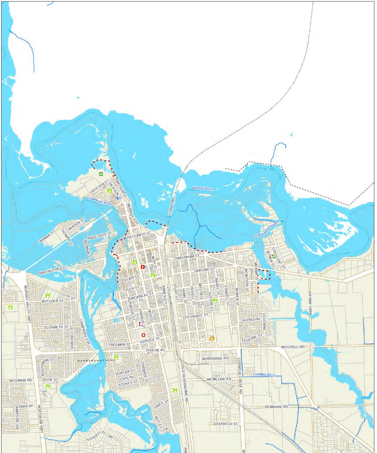
93.9m AHD at Echuca Wharf (Moderate Flood Level)
