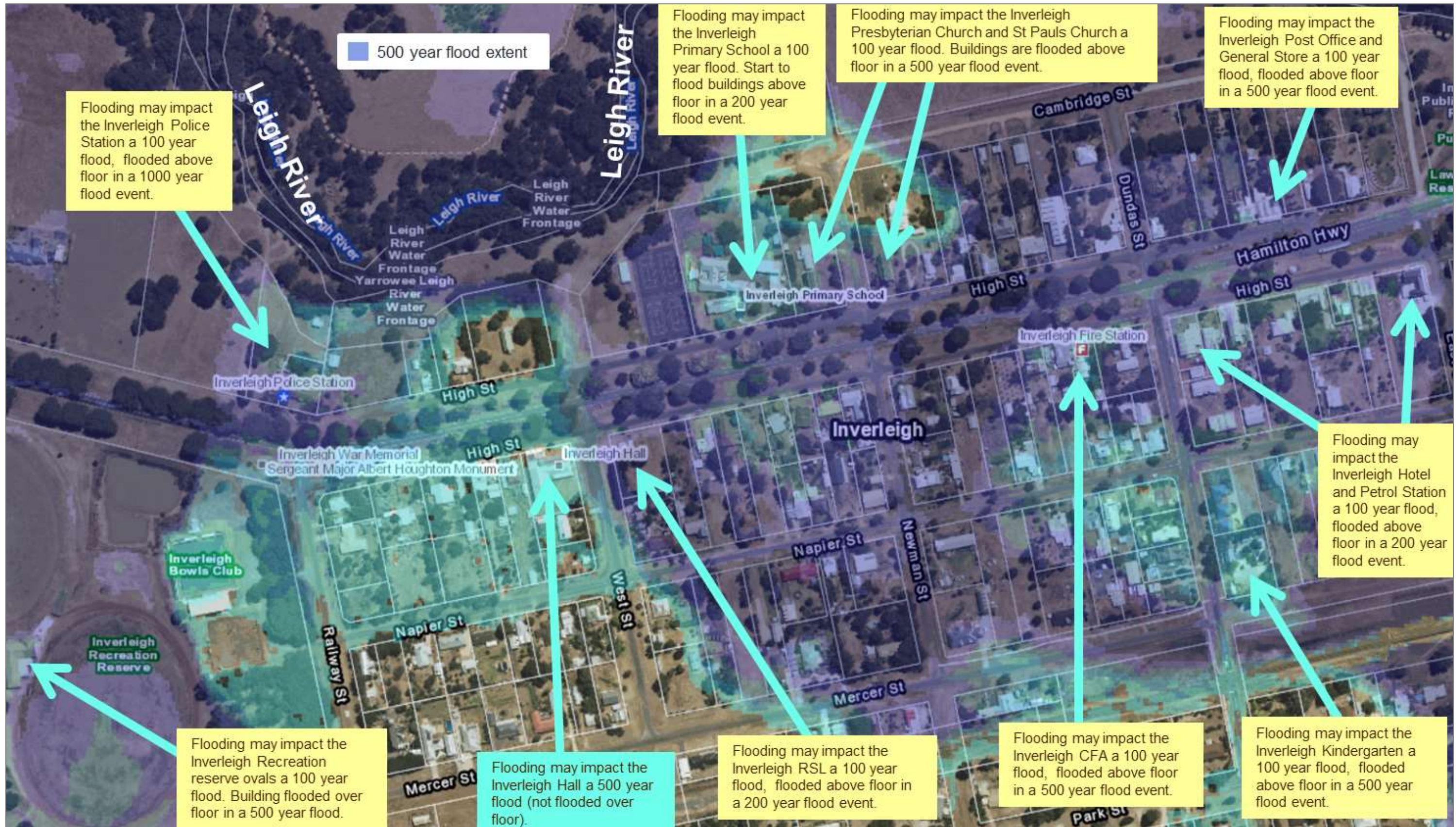
Figure 24. Inverleigh assets impacted by flooding over the 500 year flood extent (Leigh River dominant flood).
