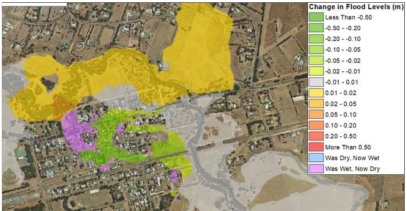
Figure 16. Changes to flood levels for flood mitigation option 1, raising the existing levee (Water Technology 2018).
