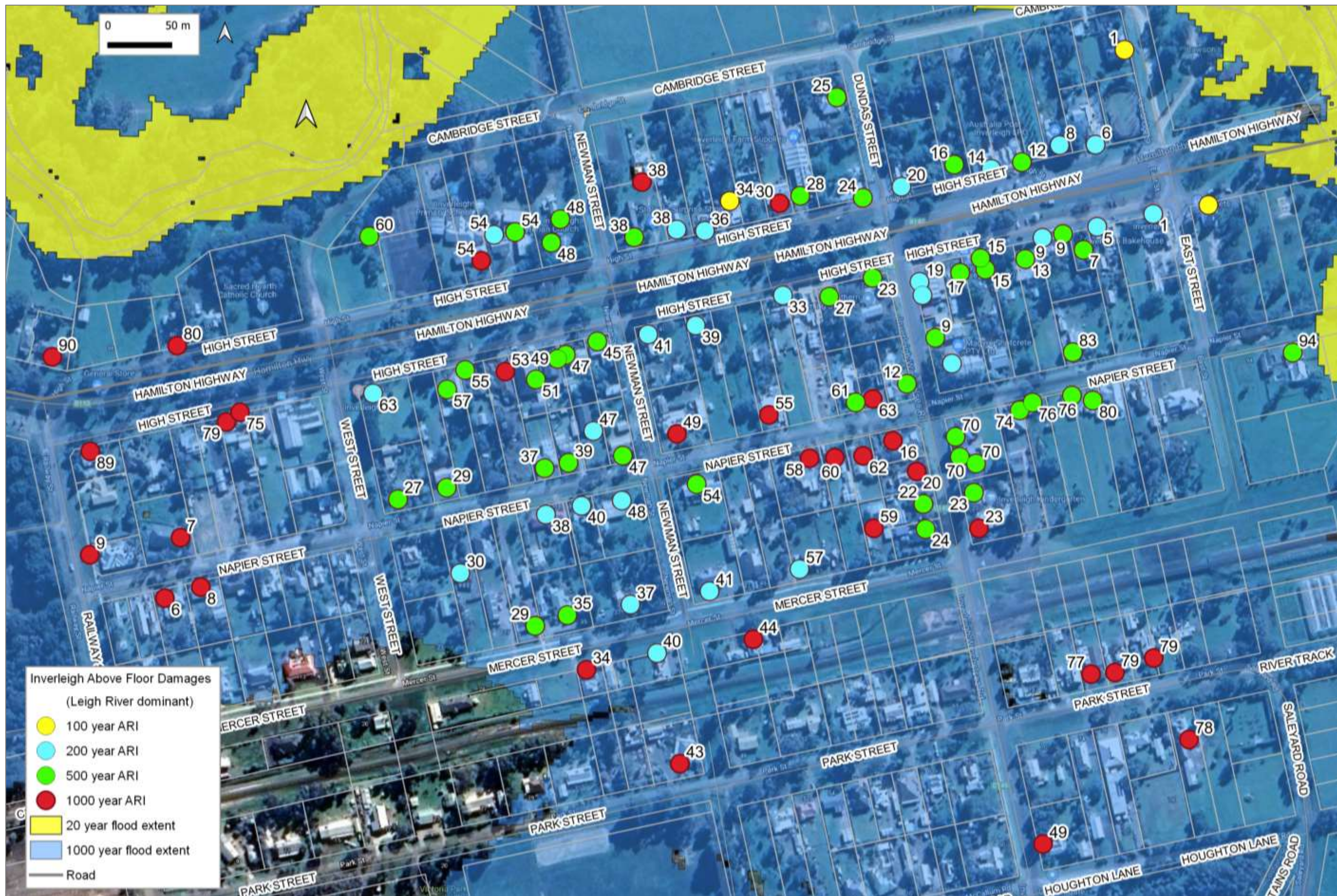
Figure 27. Inverleigh above floor damages over a range of design flood events for a Leigh River dominant flood (Water Technology 2018).
