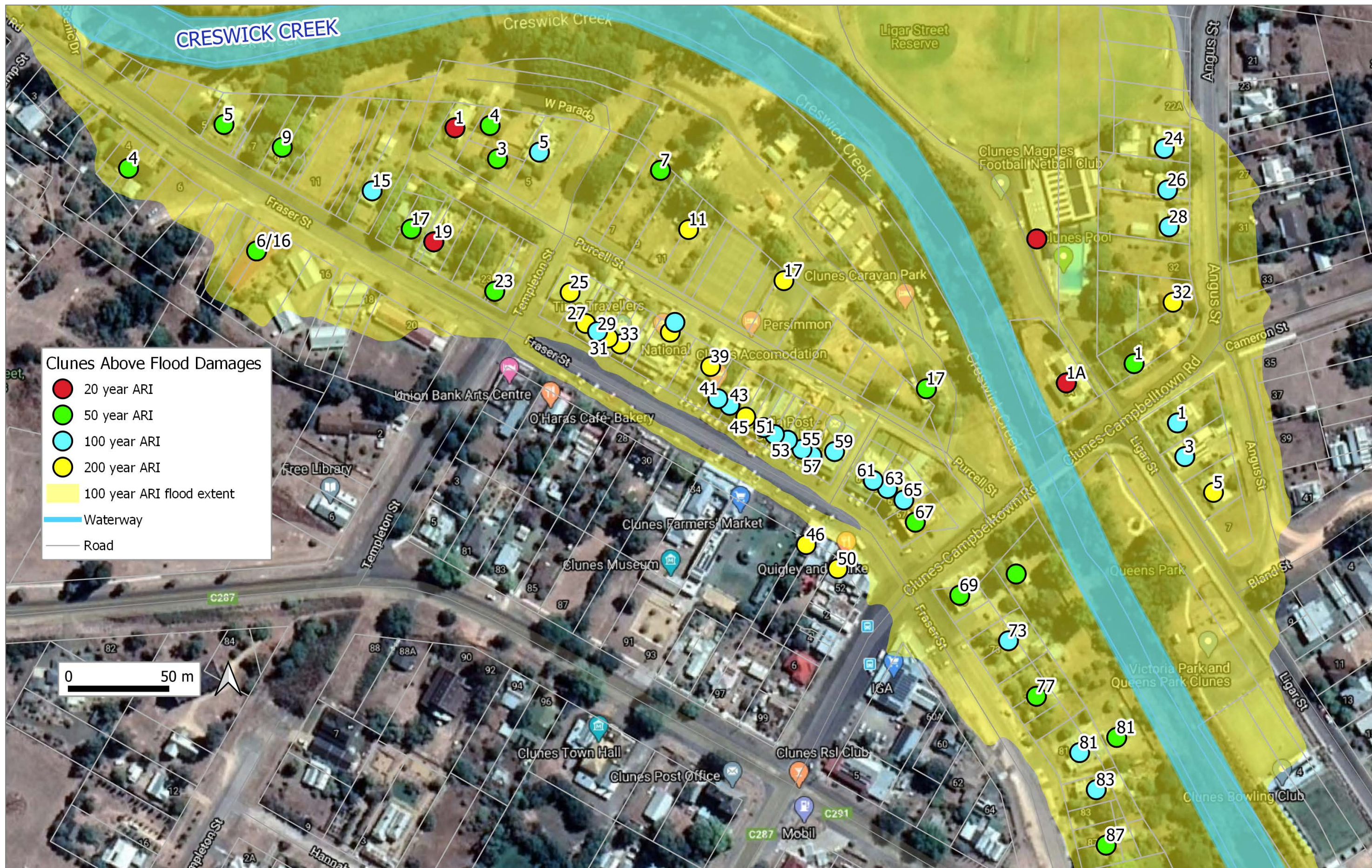
Clunes above floor building damages for a range of design flood events with the 100 year ARI flood extent (Water Technology 2012).
