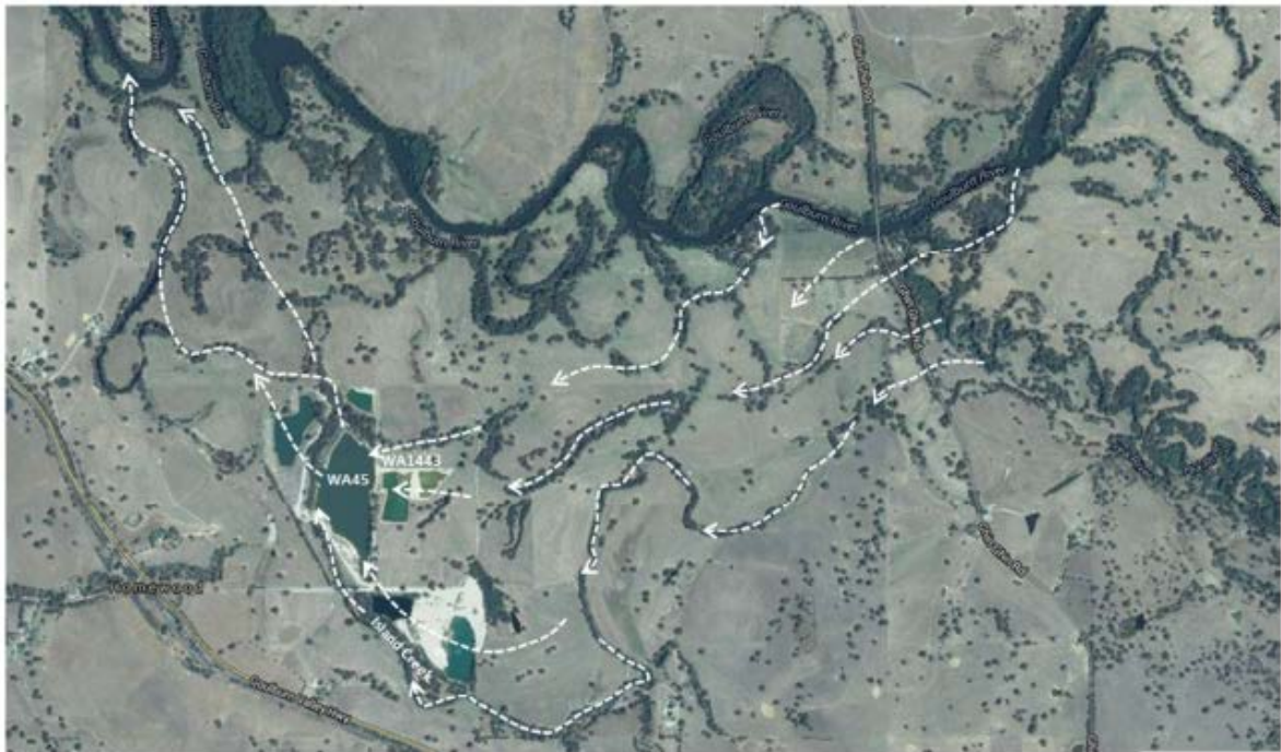
Figure 3.6: Preferred flow and potential avulsion paths and points of flow entry and exit into WA45 and WA1443 pits.
