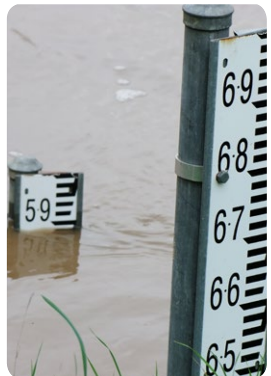
An example of a flood gauge
