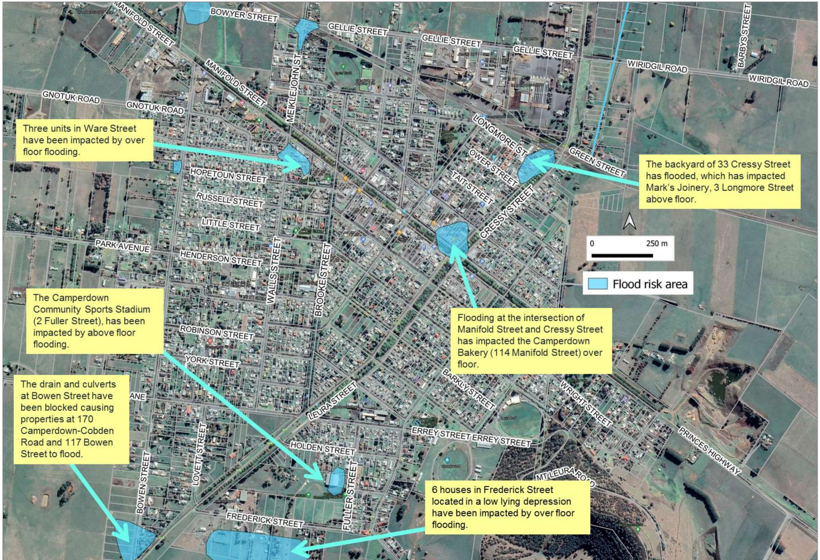
Figure 26. Area at risk of stormwater flooding in Camperdown (source VICSES Camperdown Unit).
