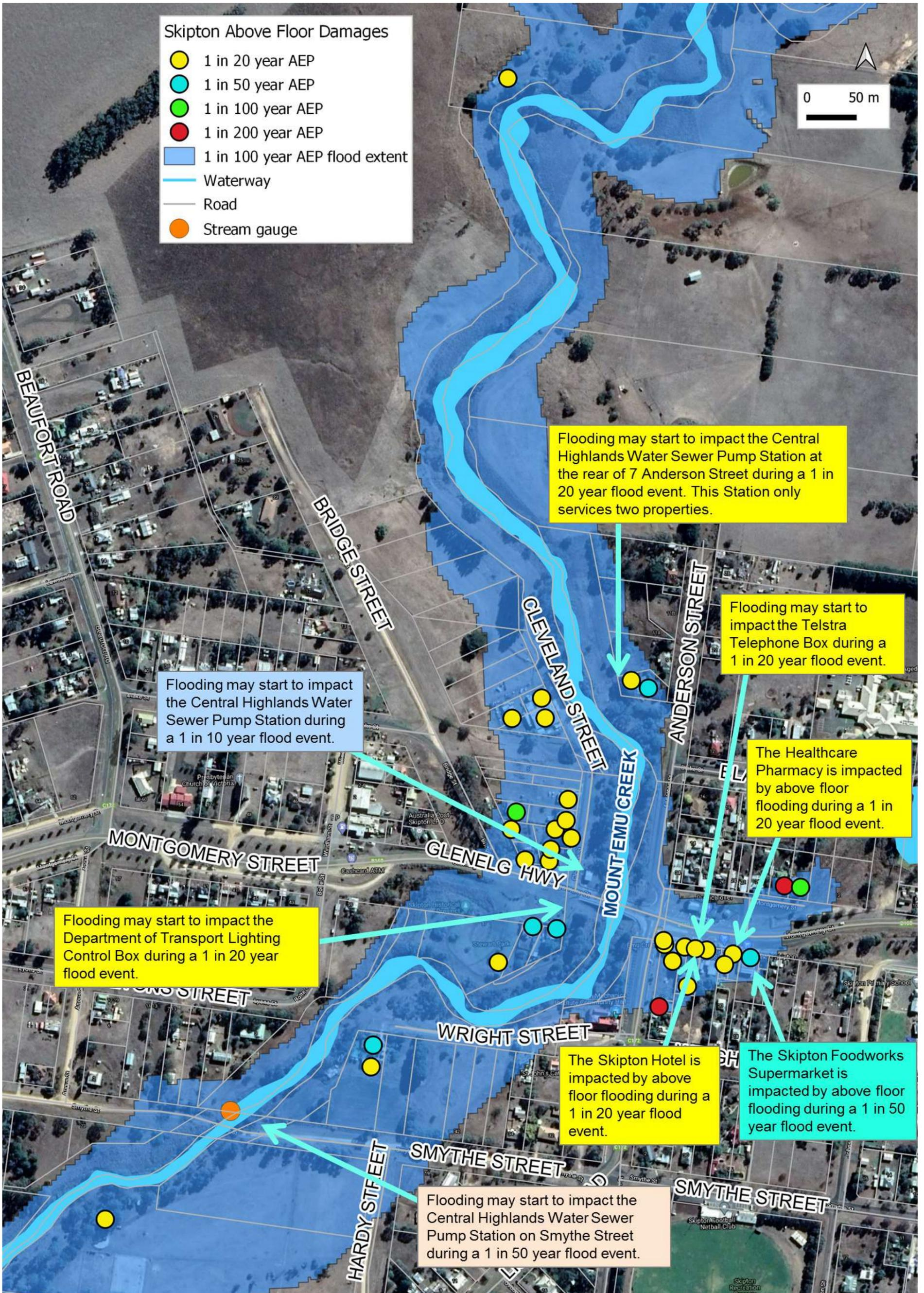
Figure 23. Skipton assets impacted by flooding with the 1 in 100 year flood extent (Water Technology 2020).
