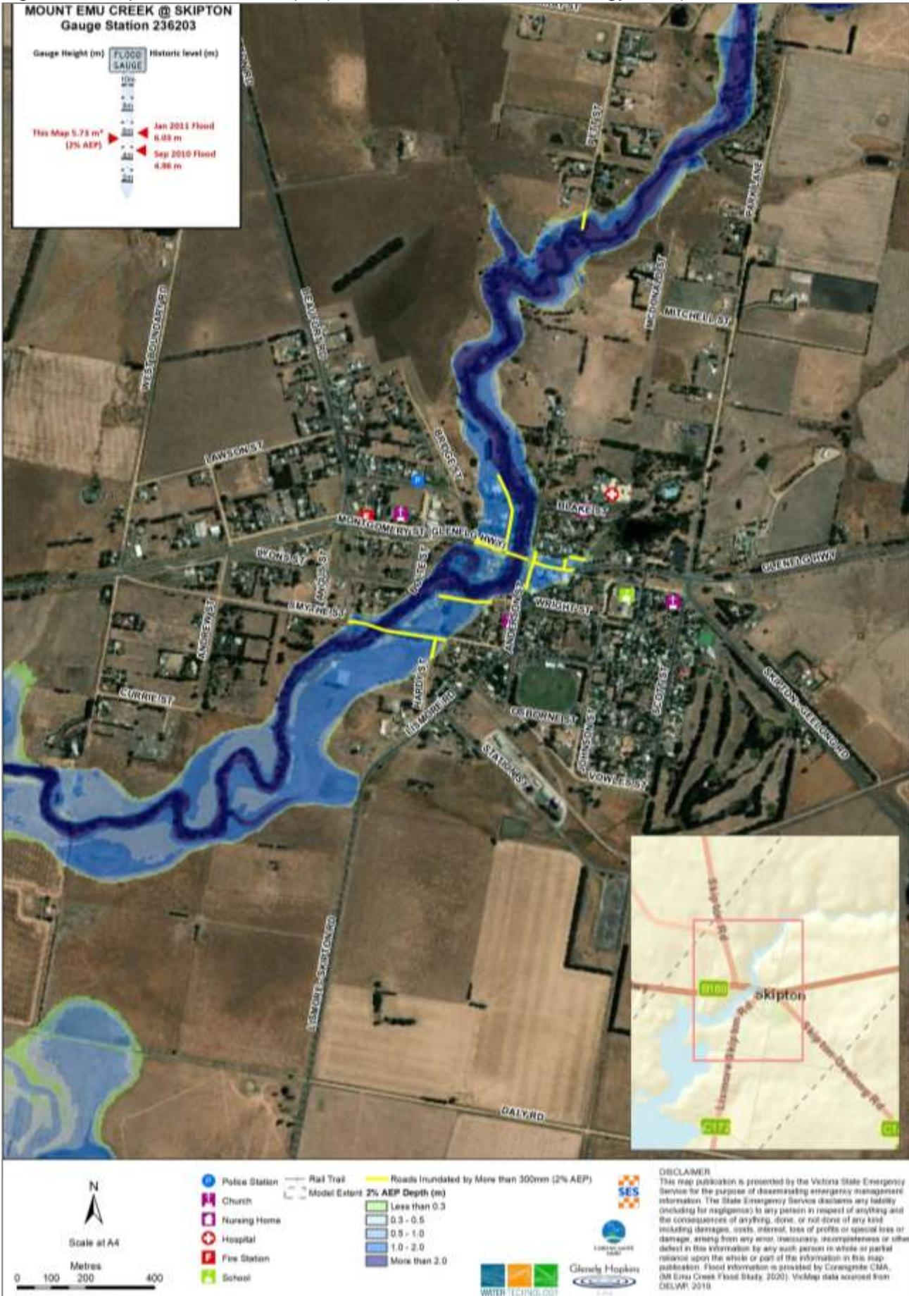
Figure 70. Skipton 1 in 100 AEP (1%) flood extent (Water Technology 2020).
