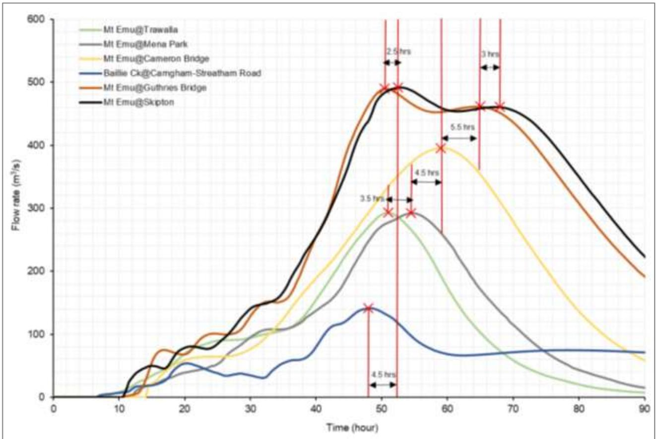
Figure 18. The travel time of flood peaks for a 1 in 100 year AEP flood, with a 48 hour duration (Water Technology 2020).
