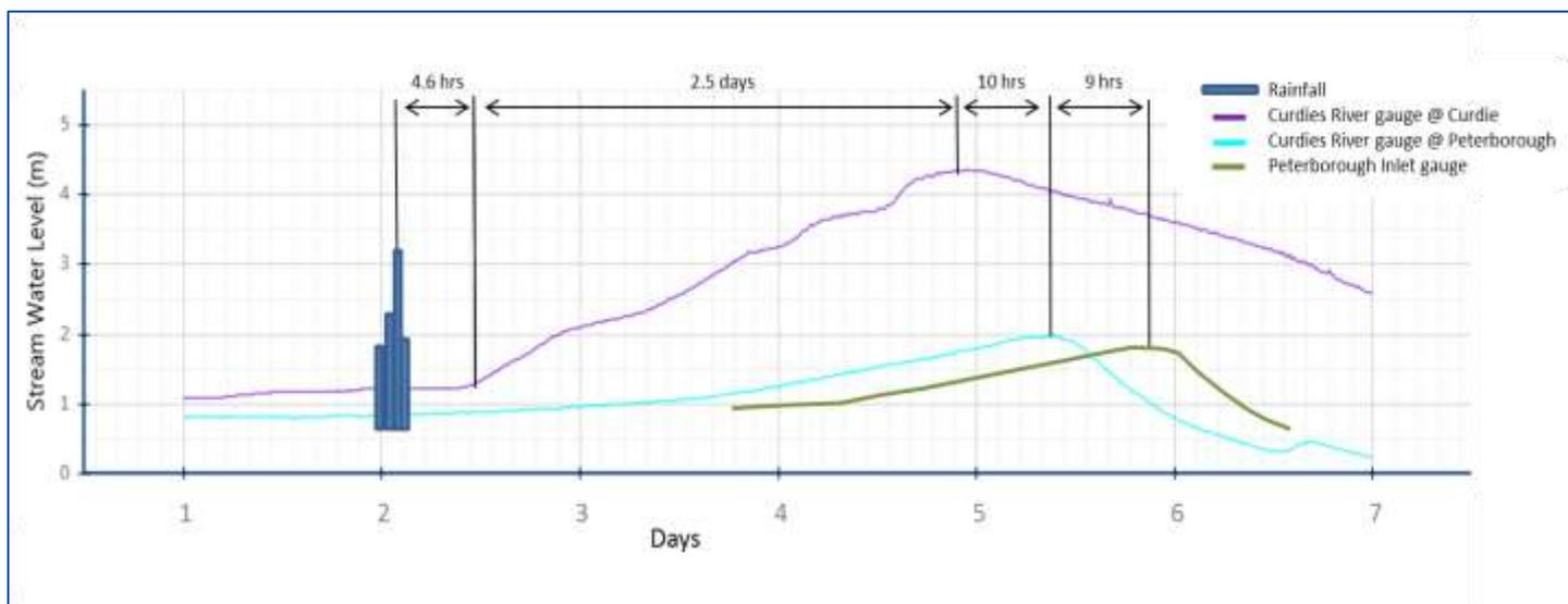
Figure 61. Curdies River flood peak travel times for a range of flood events (Corangamite CMA).
