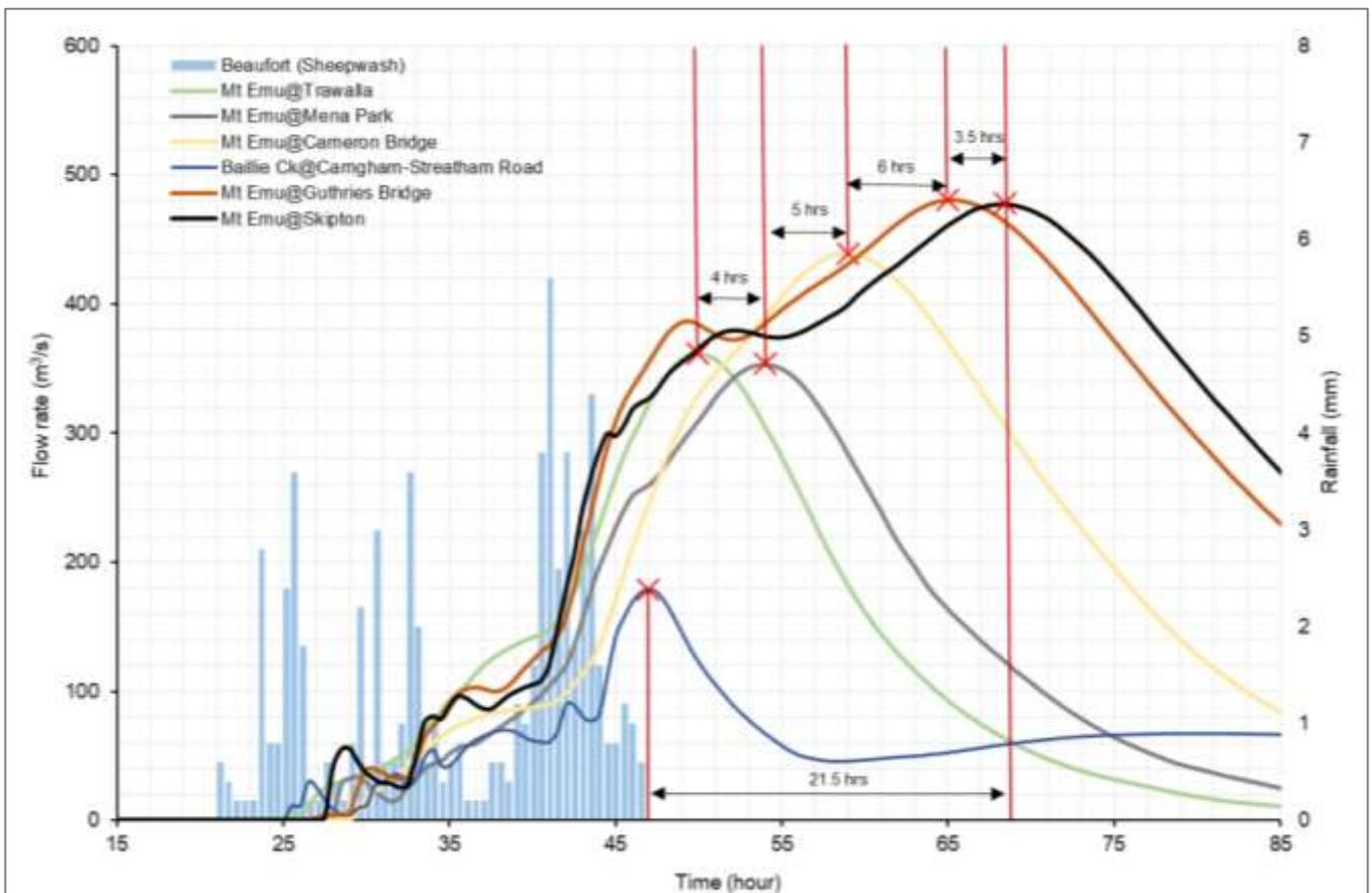
Figure 16. The travel time of flood peaks during the January 2011 flood event (Water Technology 2020).
