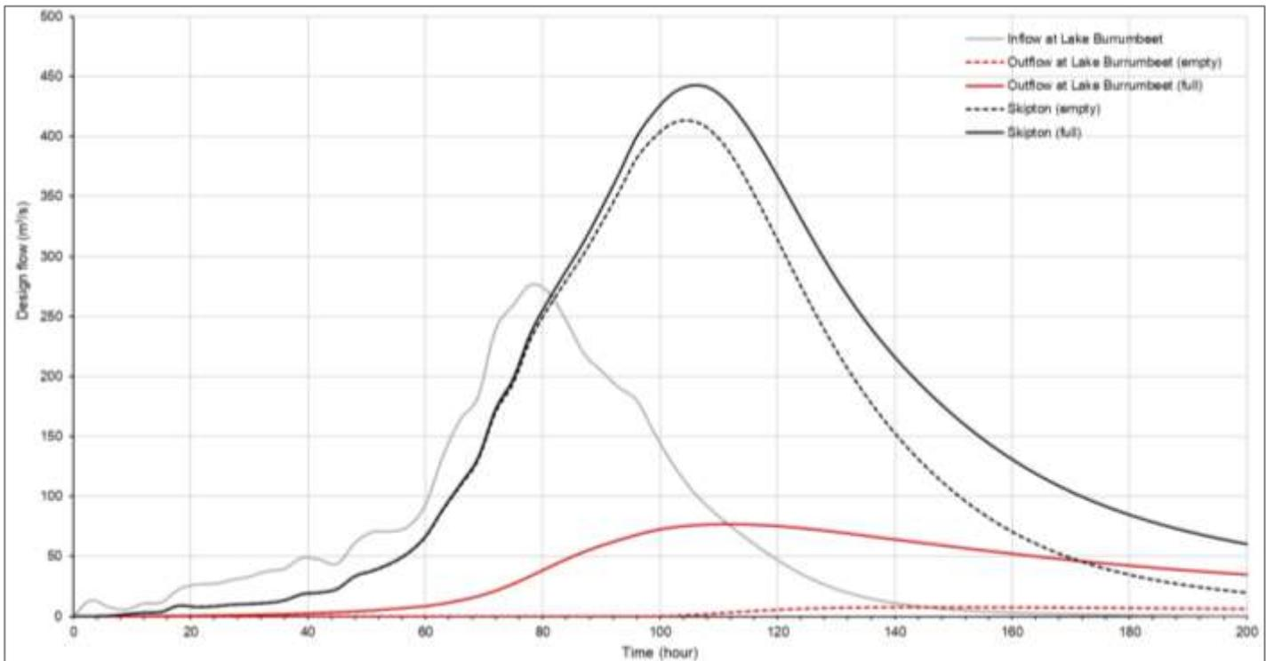
Figure 13. Sensitivity test on initial Lake Burrumbeet Storage. Stream gauge locations upstream of Dimboola.
