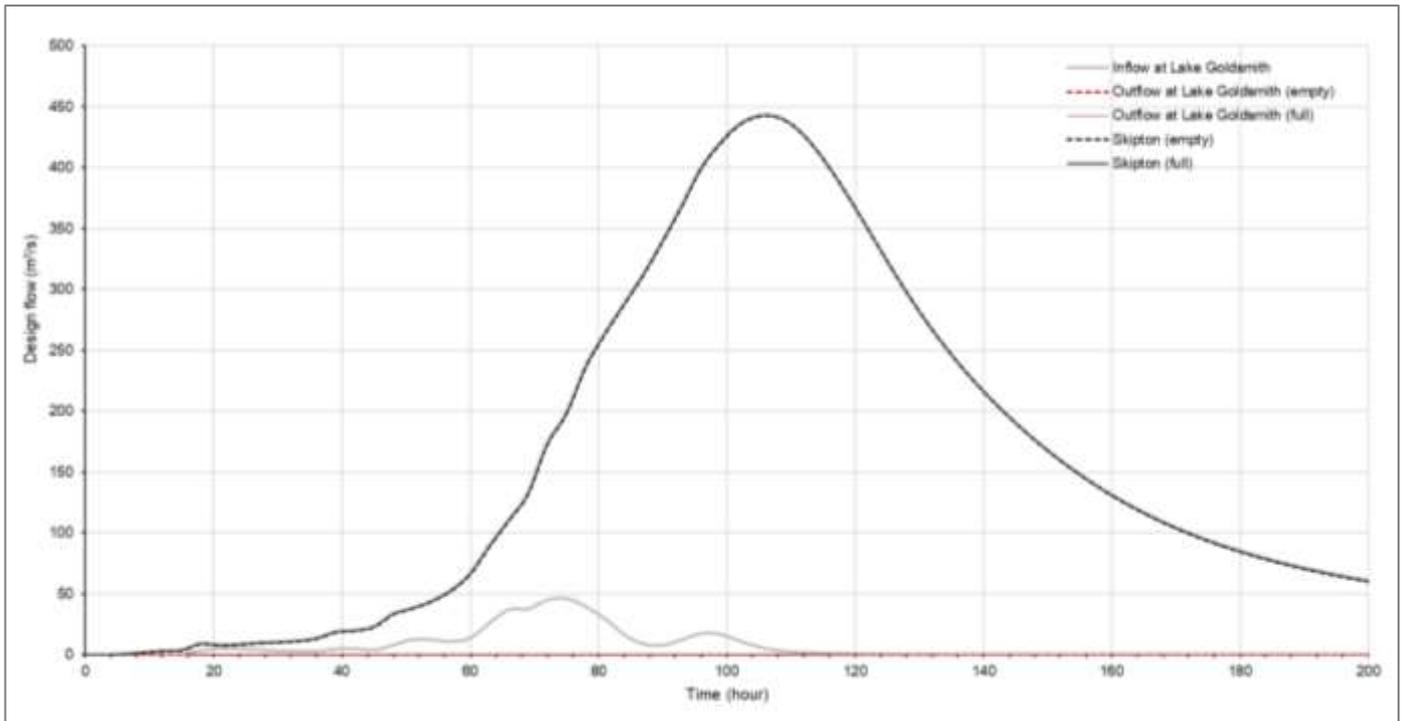
Figure 14. Sensitivity test on initial Lake Goldsmith Storage.
