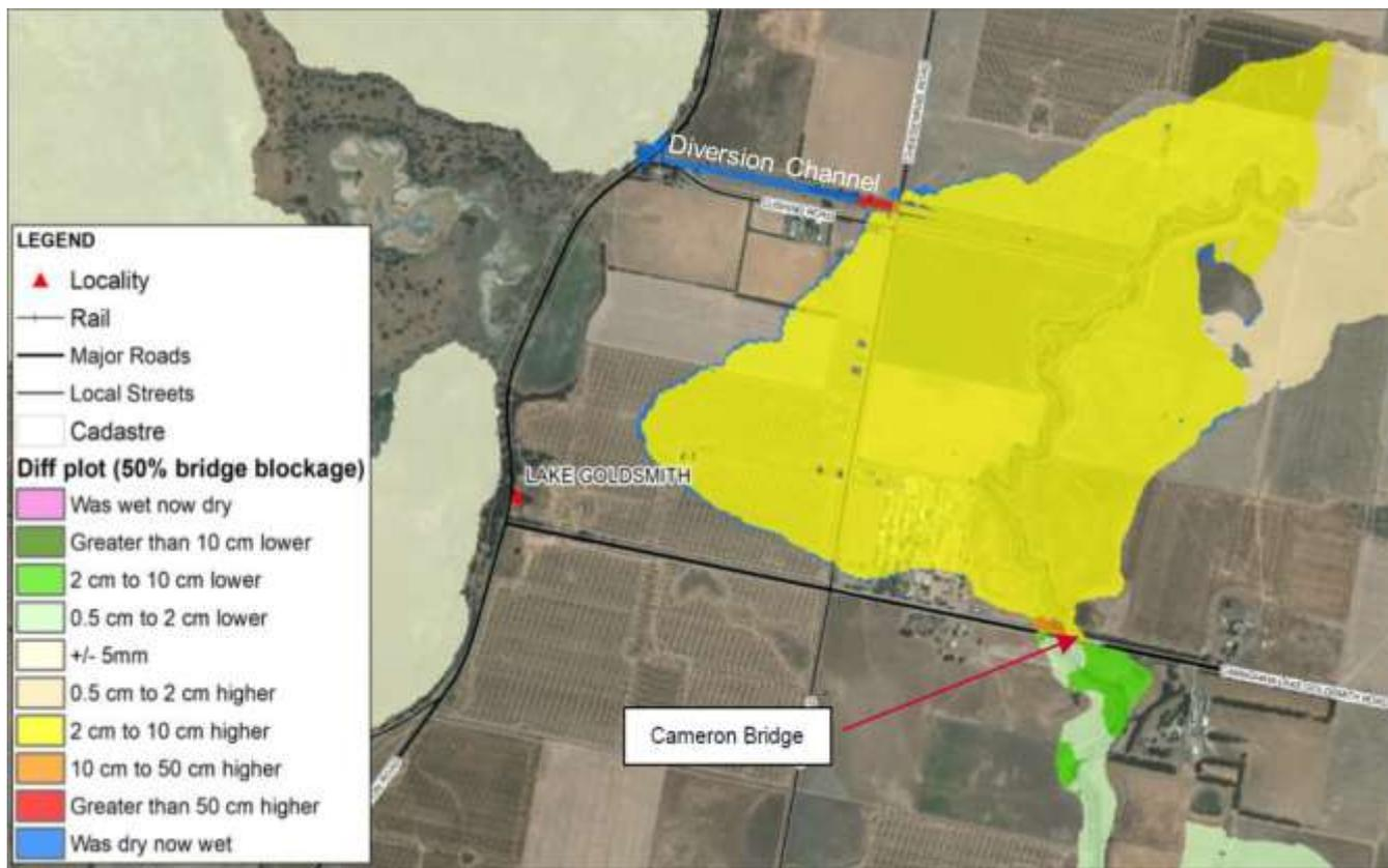
Figure 15. Modelling analysis of a blockage at Cameron Bridge at Lake Goldsmith.
