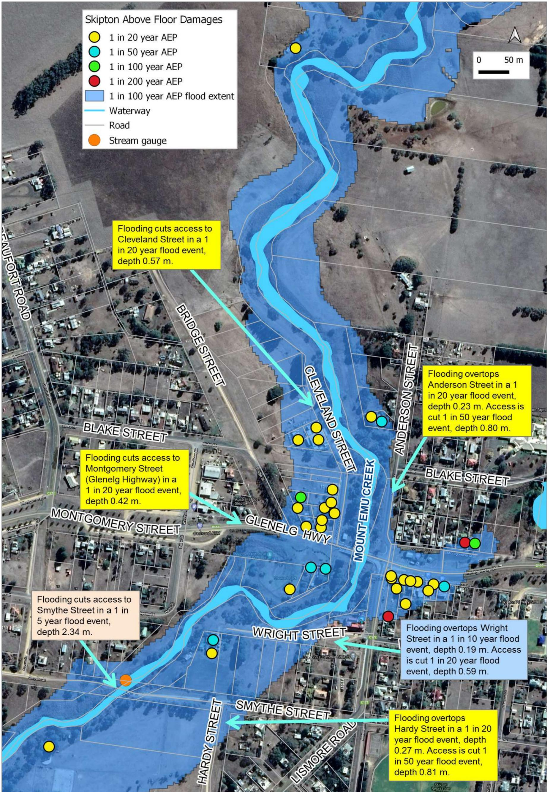
Figure 24. Skipton roads impacted by flooding with the 1 in 100 year flood extent (Water Technology 2020).
