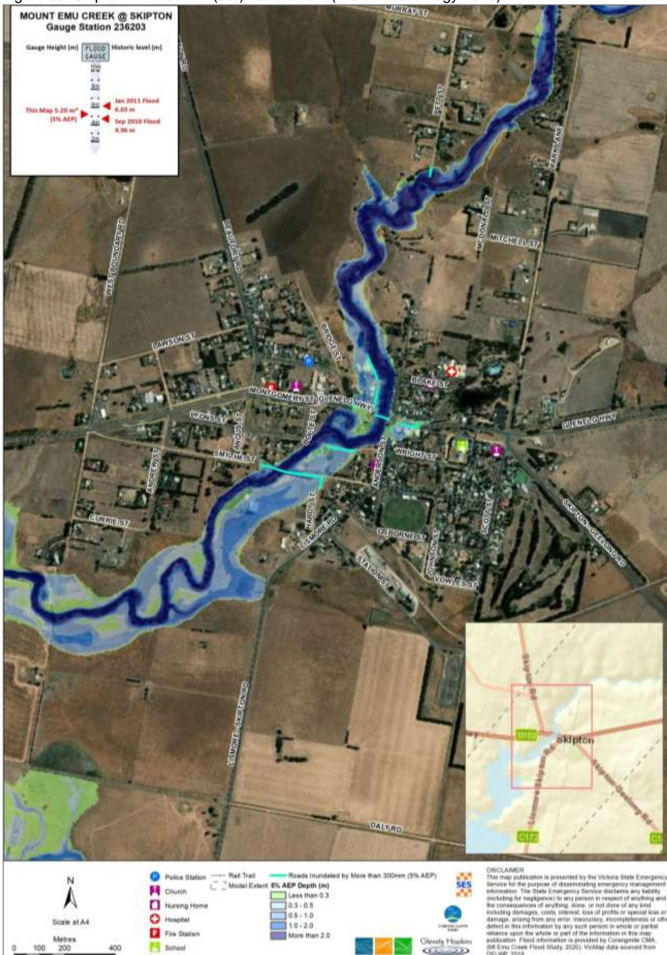
Figure 69. Skipton 1 in 50 AEP (2%) flood extent (Water Technology 2020).
