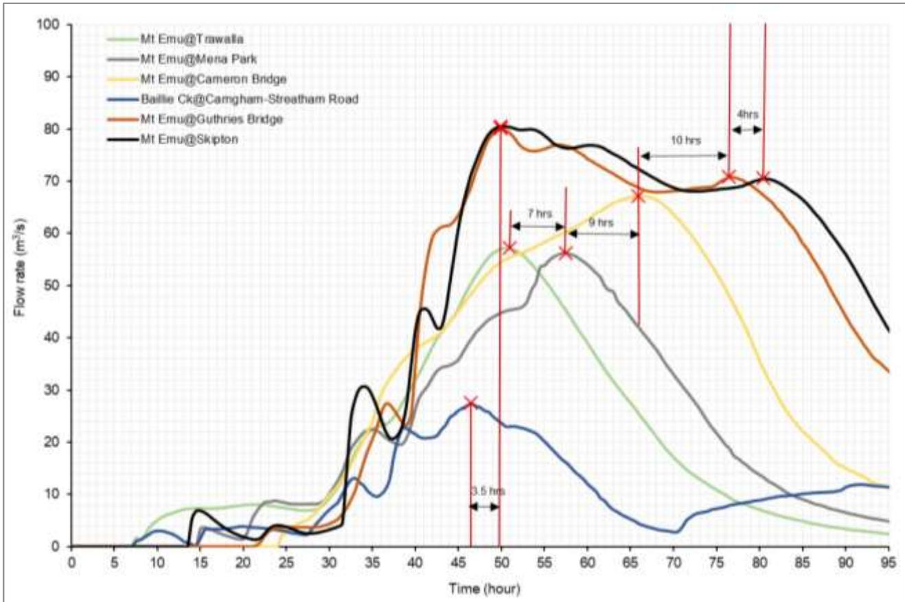
Figure 19. The travel time of flood peaks for a 1 in 20 year AEP flood, with a 48 hour duration (Water Technology 2020).
