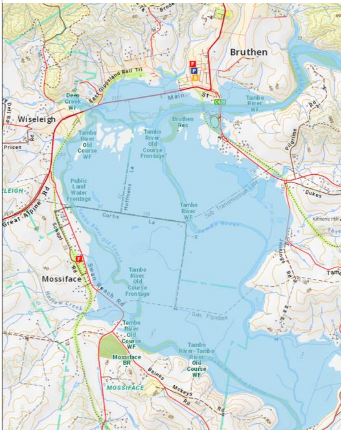
Flood extent for a gauge height 11.9m (a 1% flood extent) in the Bruthen area.
