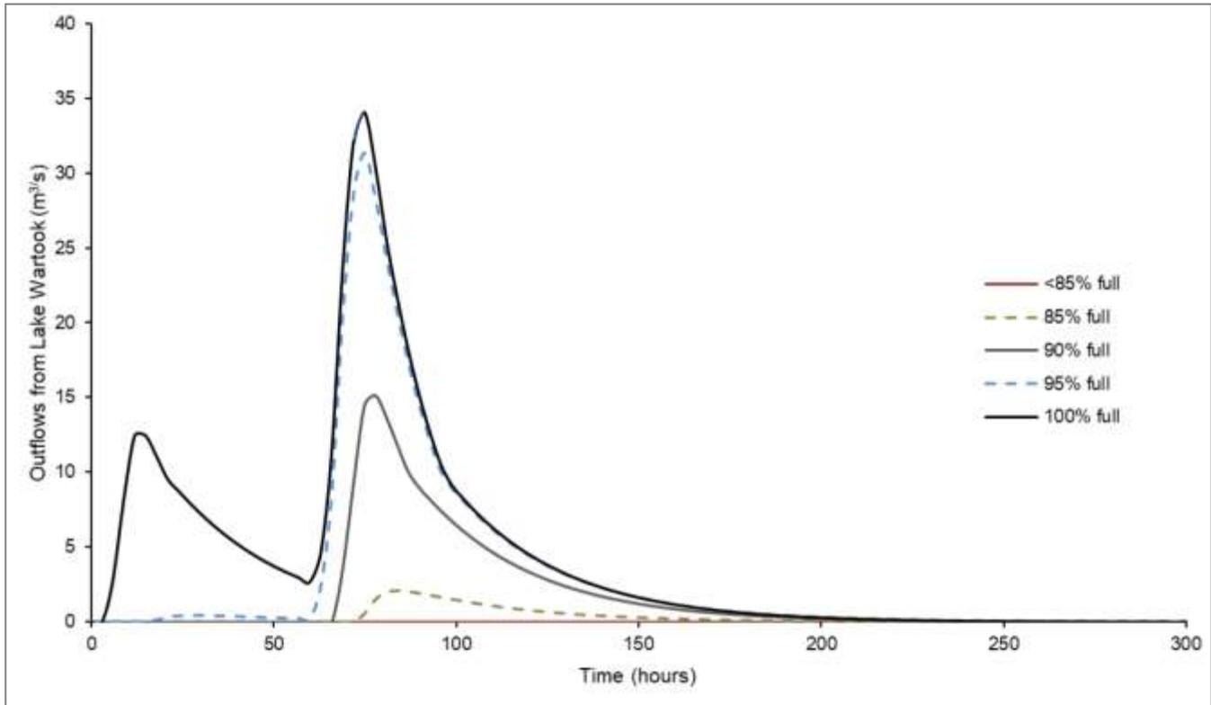
Figure 9. The impact of increasing the Lake Wartook water level during a 72 hour storm event (Water Technology 2019).
