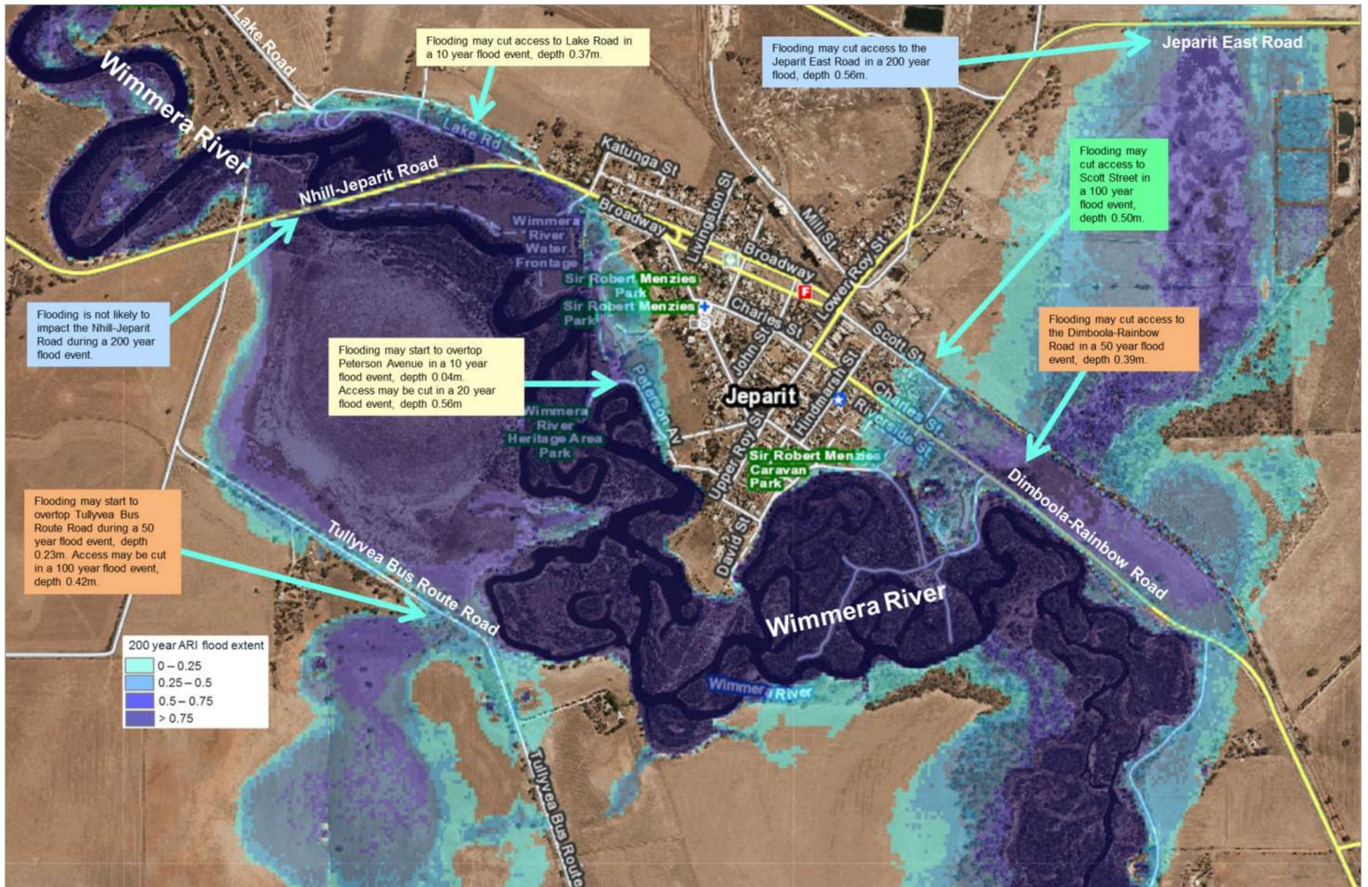
Figure 50. Jeparit roads impacted by flooding with the 200 year ARI flood extent (Water Technology 2017).
