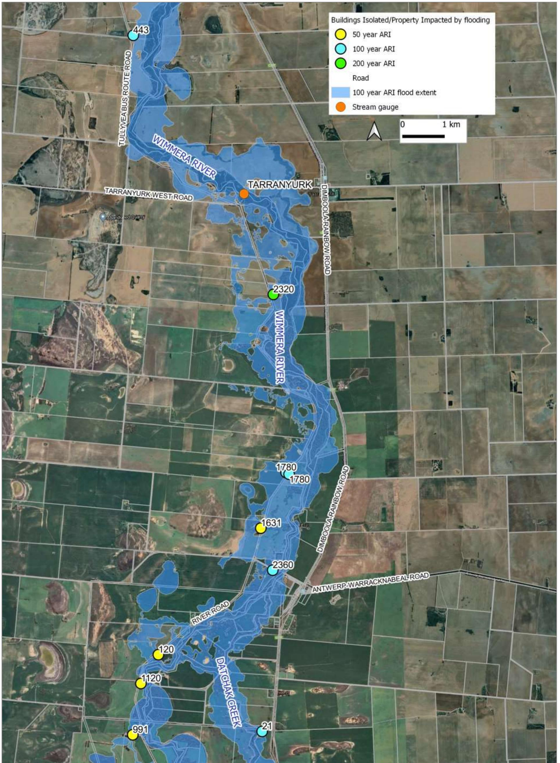
Figure 52. Buildings or properties impacted by flooding between Arkona and Jeparit with the 100 year ARI flood extent (Water Technology 2017).
