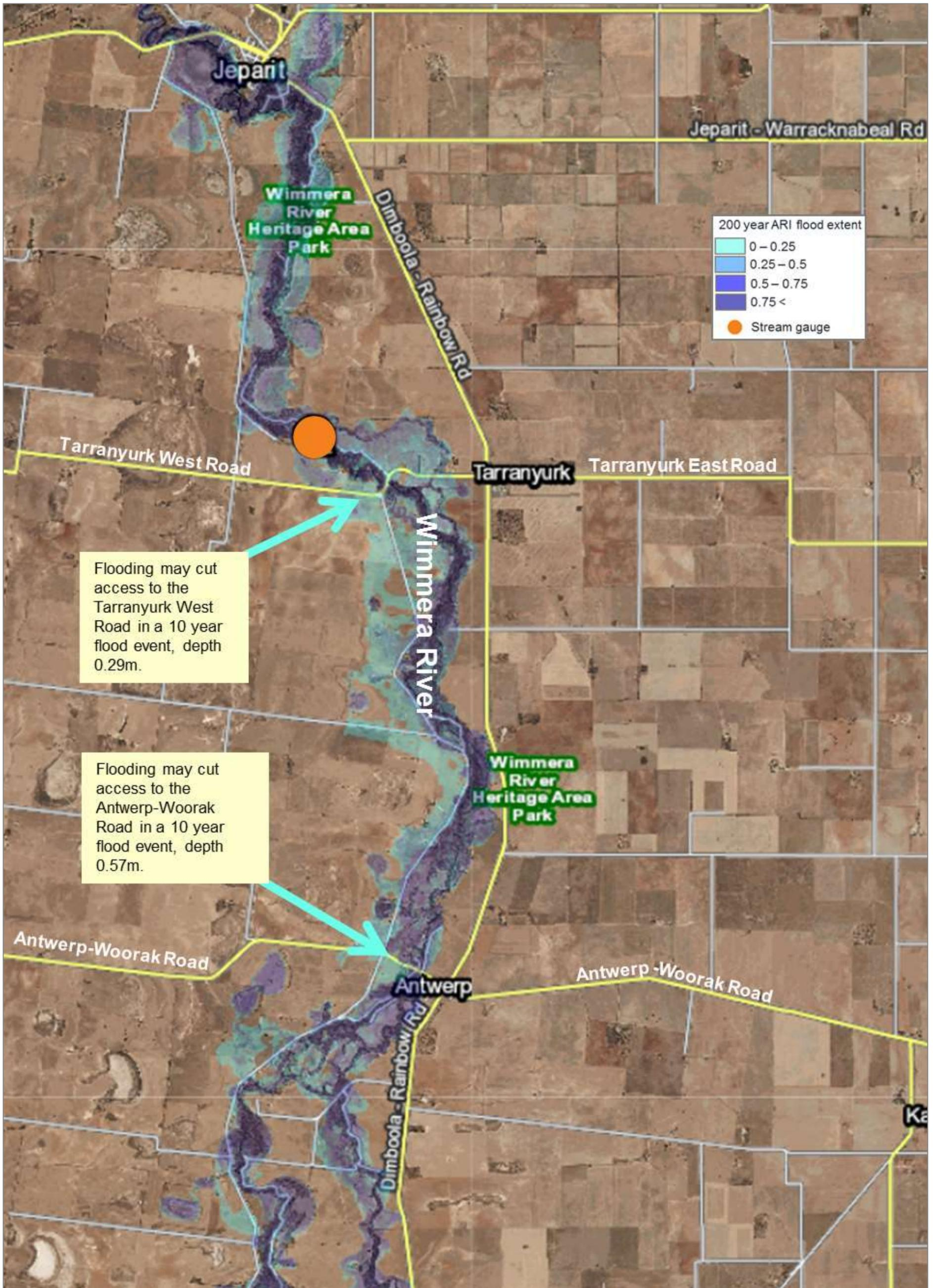
Figure 51. Roads between Arkona and Jeparit impacted by flooding with the 200 year ARI flood extent (Water Technology 2017).
