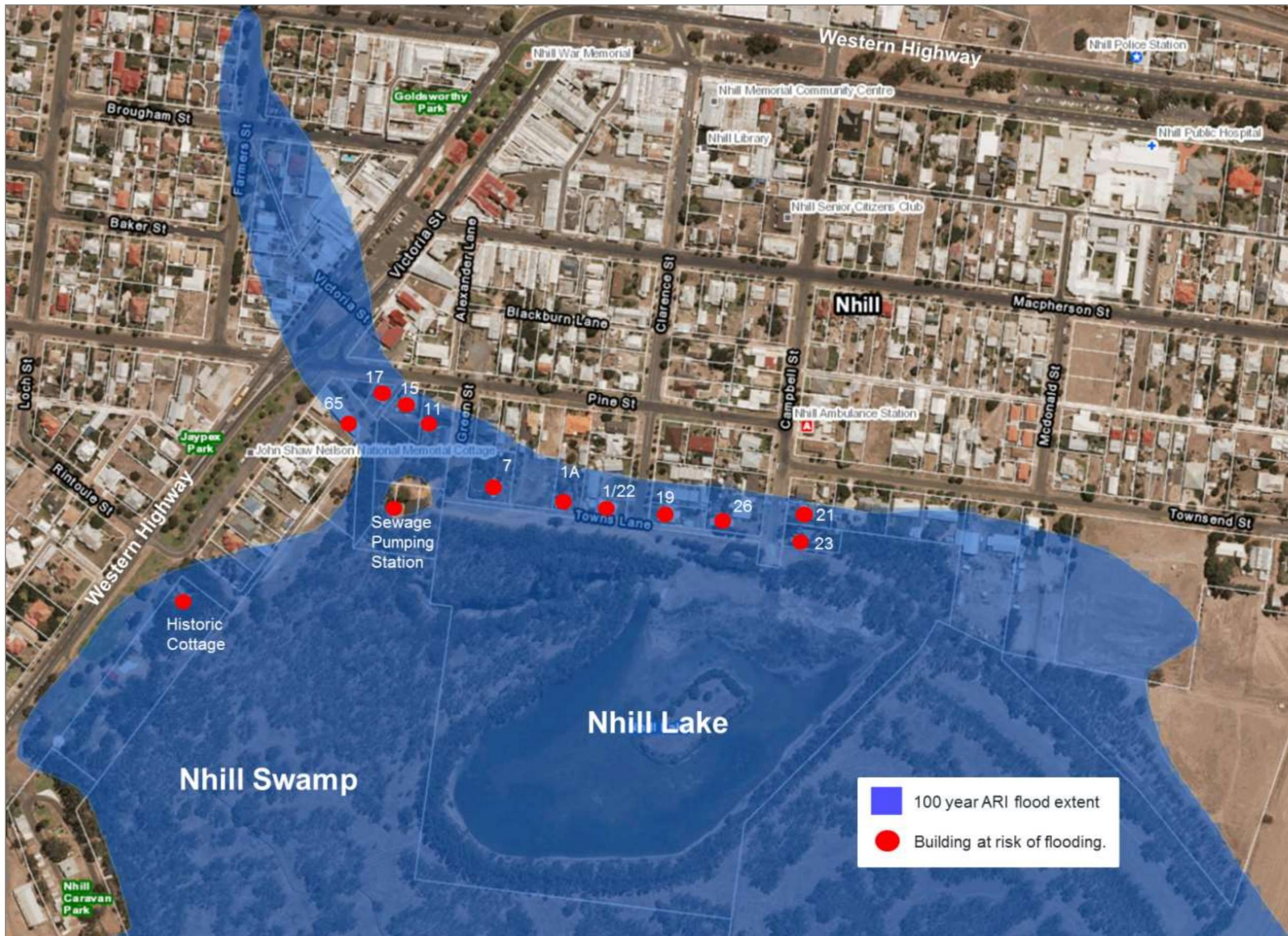
Figure 57. Nhill assets impacted by flooding with the 100 year ARI flood extent (SRWSC 1978).
