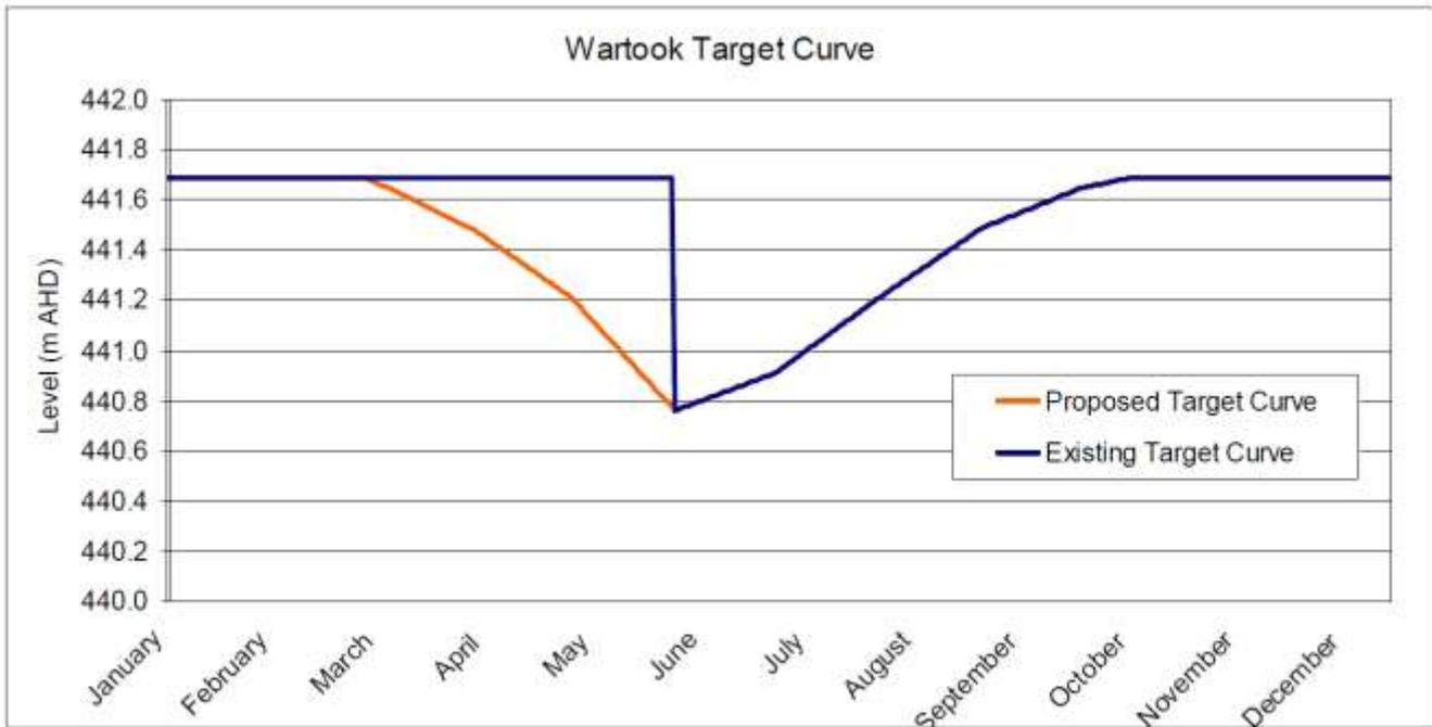
Figure 3. Lake Wartook storage level control release target curve (source GMMWater).
