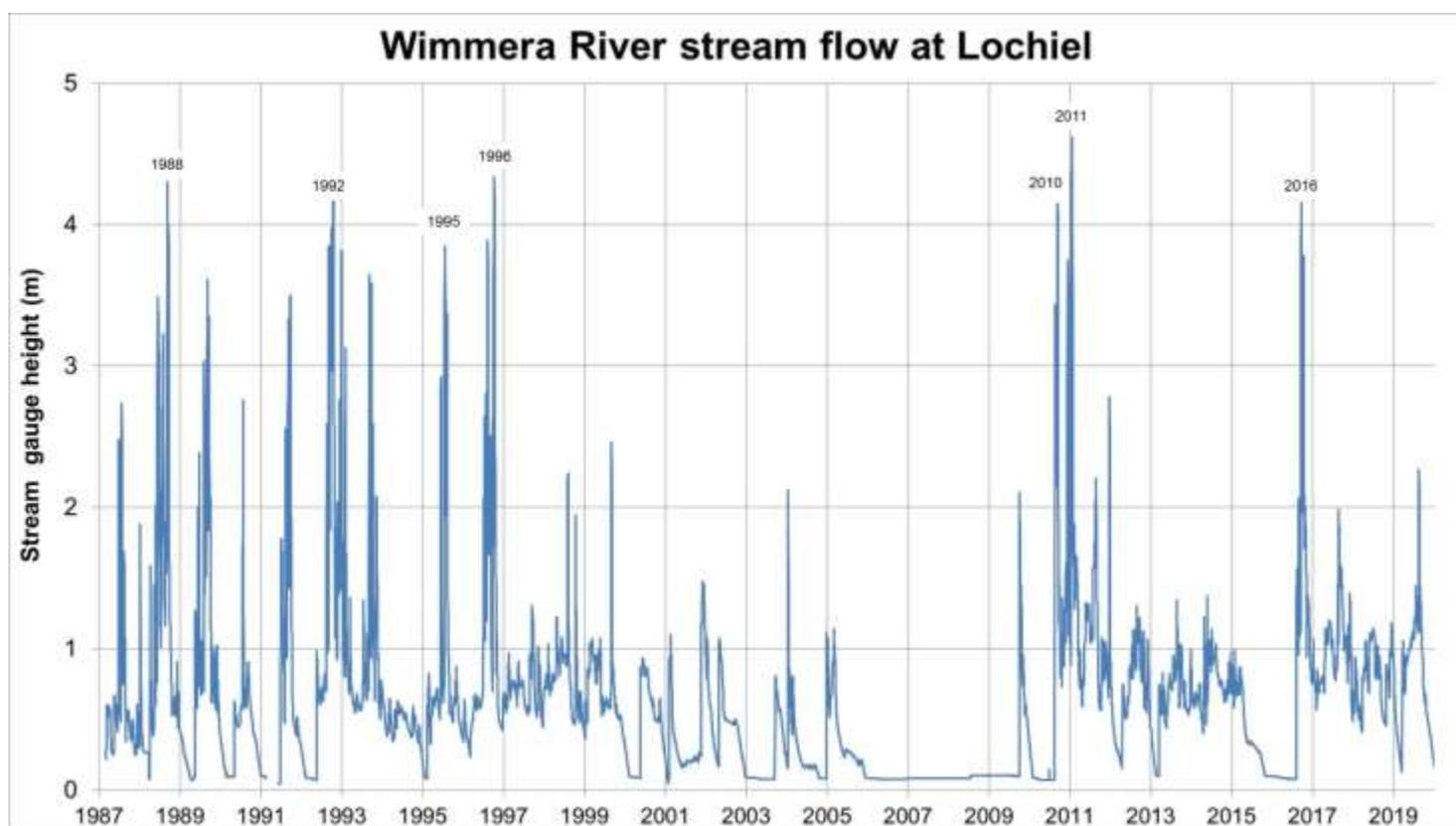
Figure 30. Wimmera River stream flow records indicate the frequency of flood events that have occurred in Jeparit.
