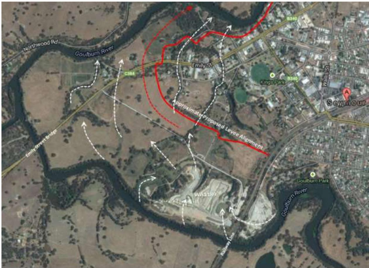
Figure 3.8: Flow and potential avulsion paths and points of flow entry and exit into pit at WA1189. The approximate proposed levee alignment is also shown.
