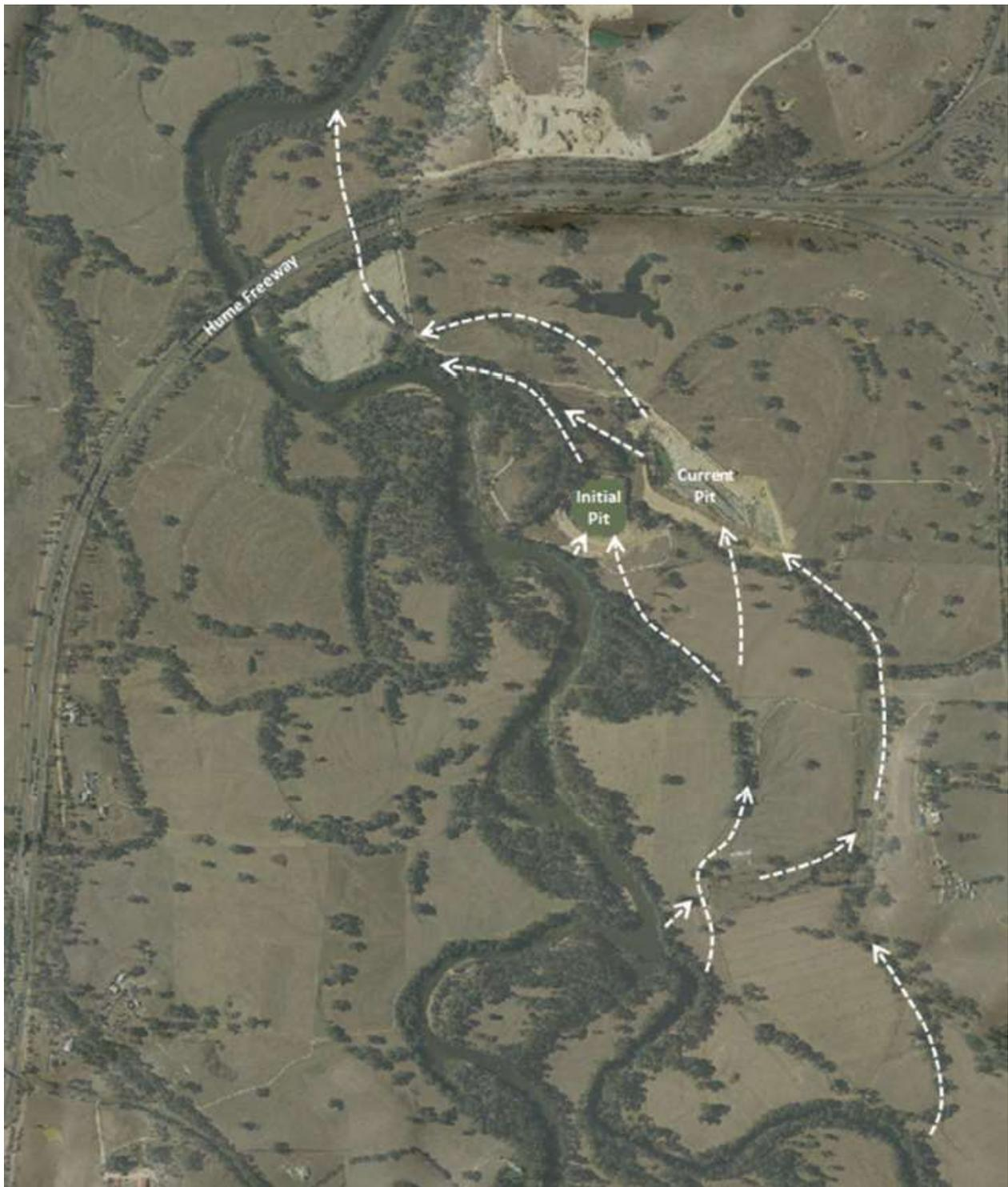
Figure 3.10: Preferred flow and potential avulsion paths and points of flow entry and exit into two pits at WA781.
