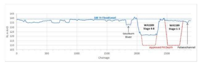
Figure 3.9: Floodplain cross-section from LiDAR showing the relief of the Goulburn River Floodplain, WA1189 Current and Approved Pits.
