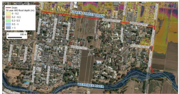
Figure 32. Floodwater breaking out from McGrath Street during a 50 year ARI flood (GHD 2010).
