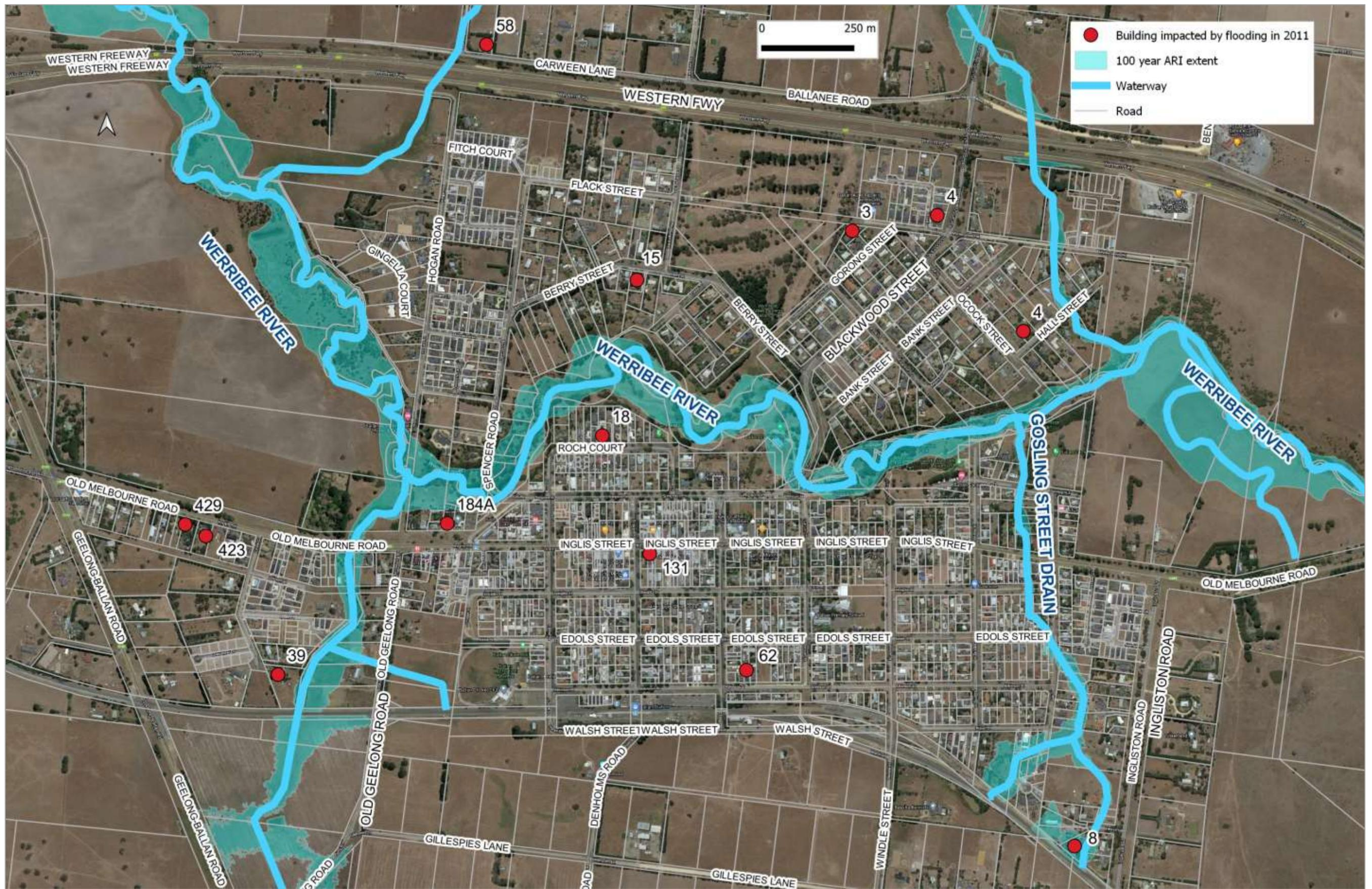
Figure 61. Buildings in Ballan impacted by above floor flooding during the January 2011 flood event (Melbourne Water).
