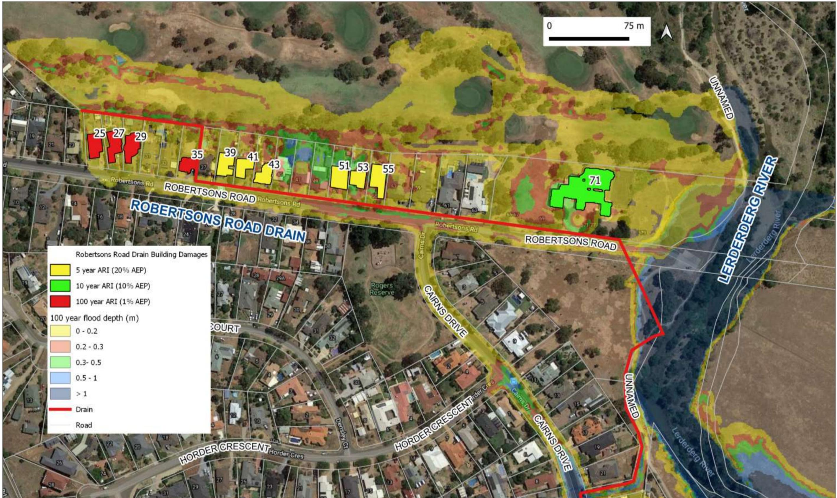
Figure 18. Buildings impacted by above floor flooding from the Robertsons Road Drain over a range of design flood events (Engeny 2011).
