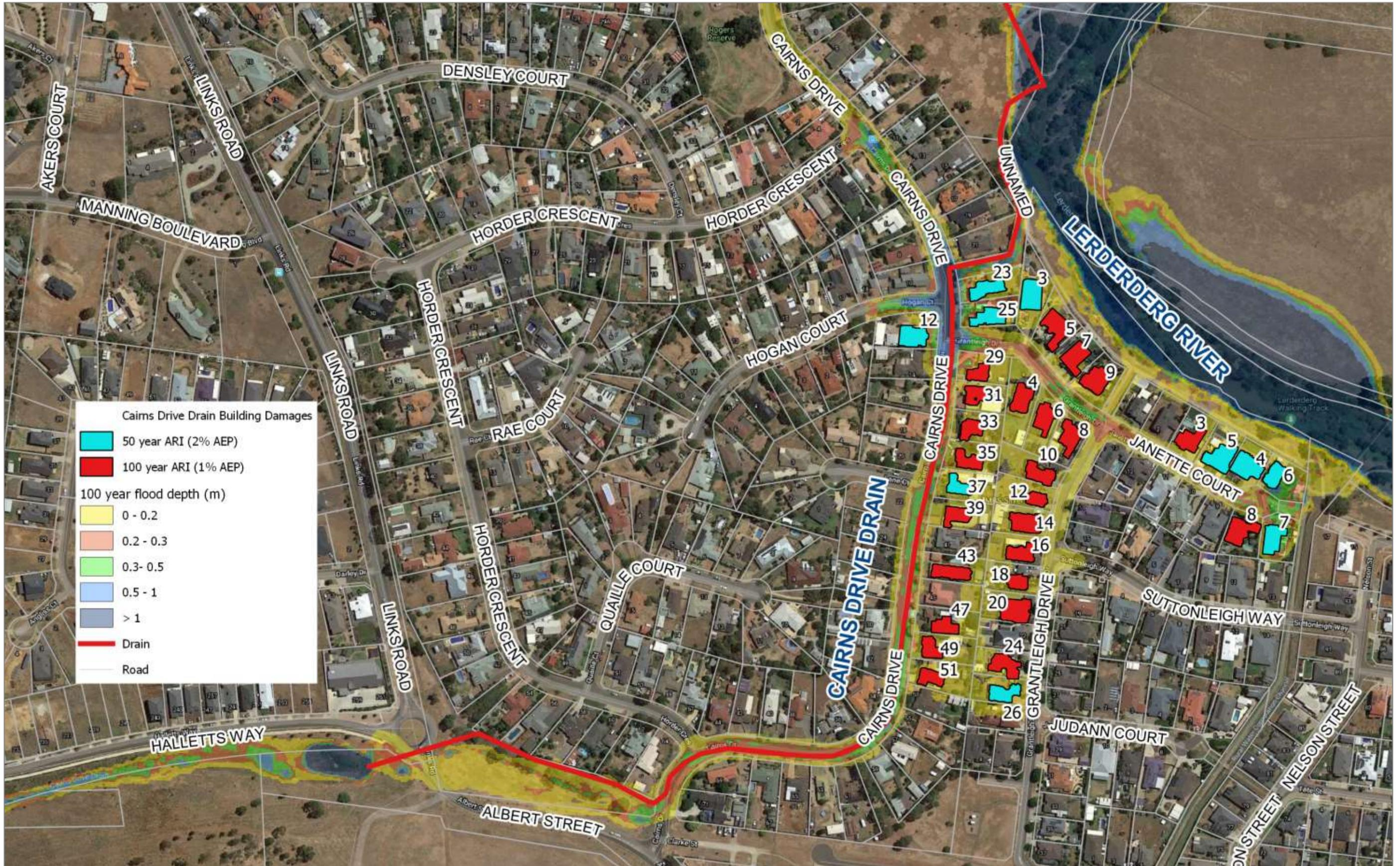
Figure 19. Buildings impacted by above floor flooding from the Cairns Drive Drain over a range of design flood events (Engeny 2011).
