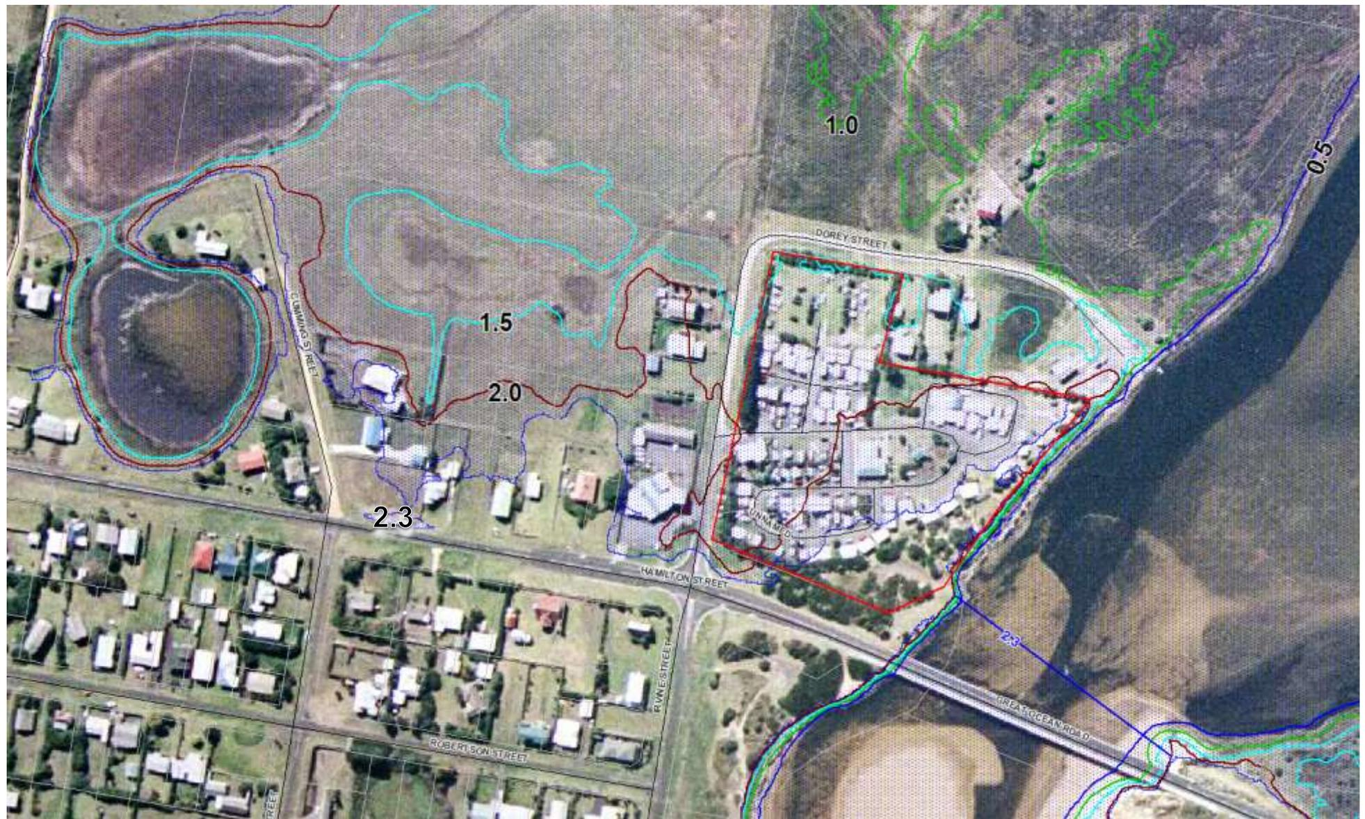
Map 1. Flood extent map, relating to the Curdies River Inlet gauge board height (m AHD), refer to the Flood Intelligence Card above. When the flood level at the Curdies River Inlet gauge board reaches 1.5 m, floodwater will extend to the light blue flood extent.
