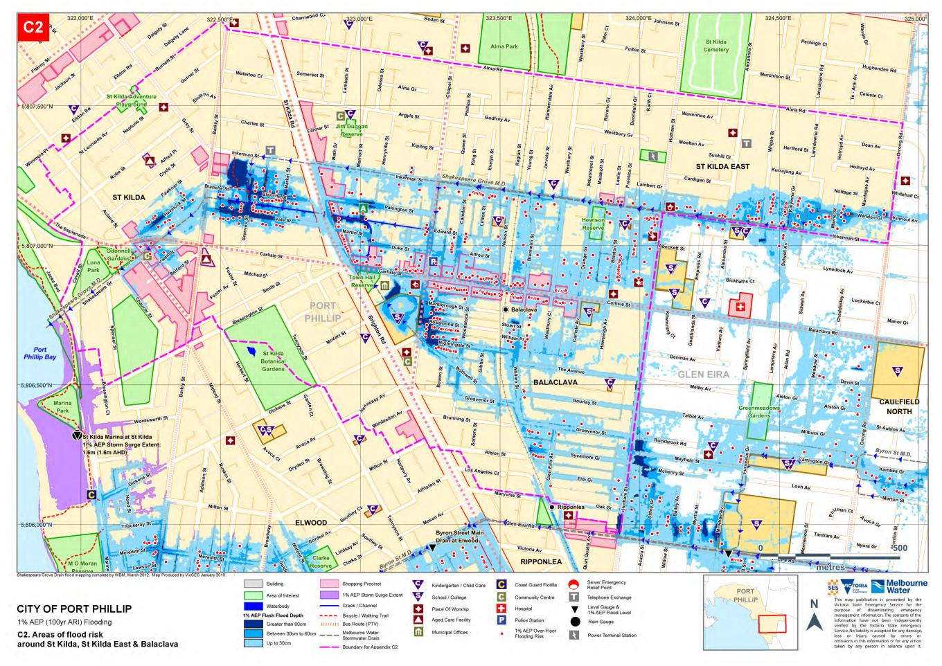
Figure C2 – Areas of flood risk along the Shakespeare Grove Drain in the City of Port Phillip
