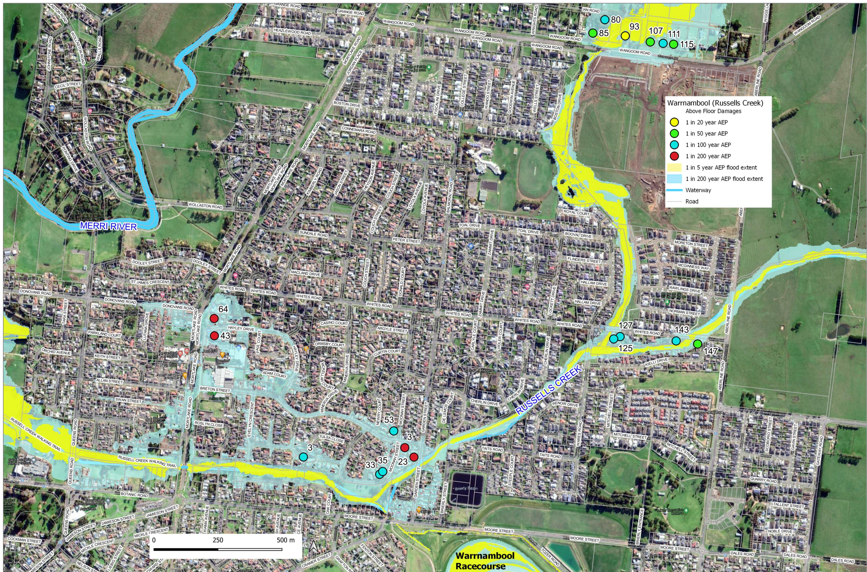
Figure 20. Warrnambool (Russells Creek) buildings impacted by over flood flooding for a range of design flood events (Water Technology 2017).
