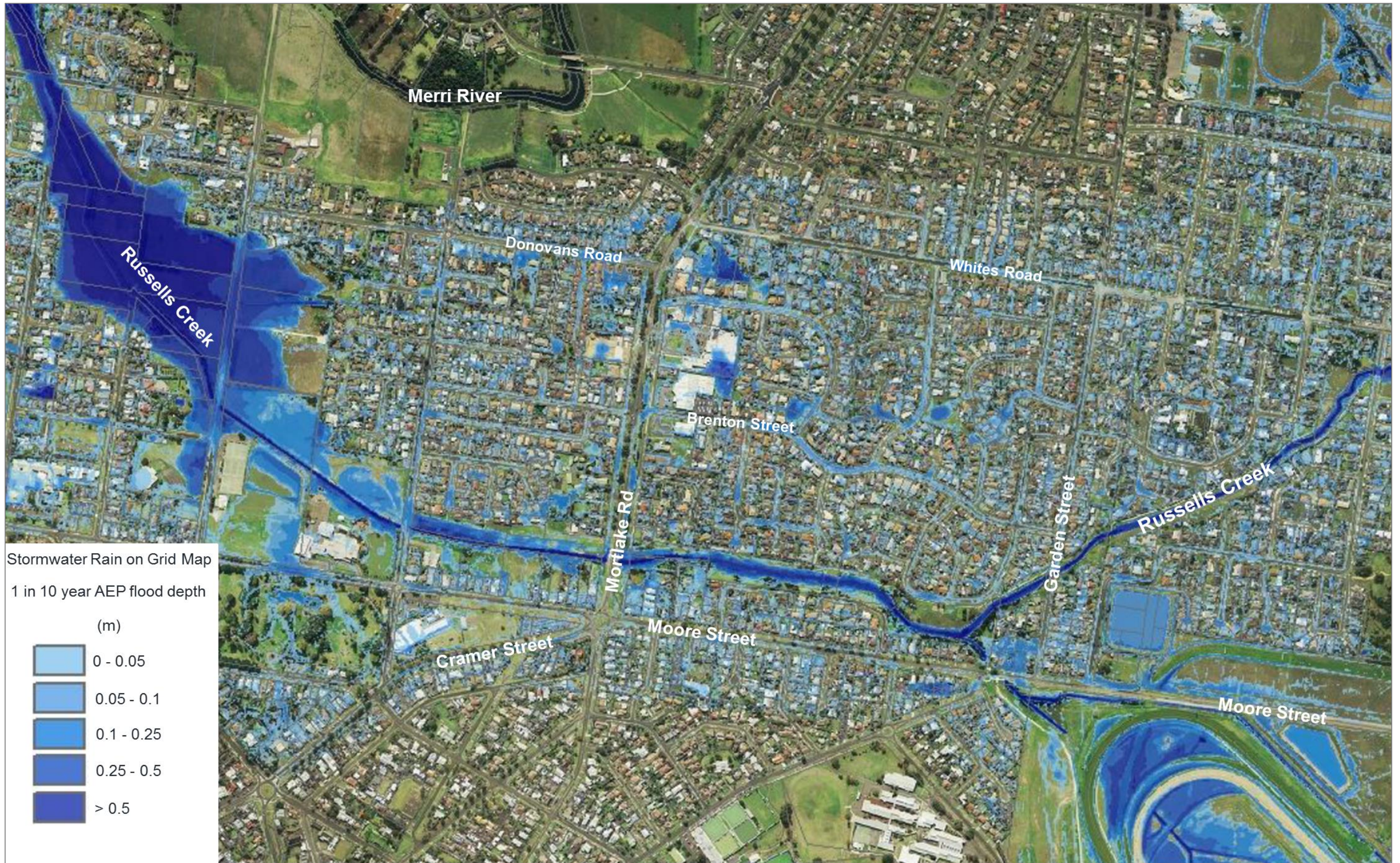
Figure 10. Areas in Warrnambool impacted by stormwater flooding during a 1 in 10 year AEP event (Water Technology 2017).
