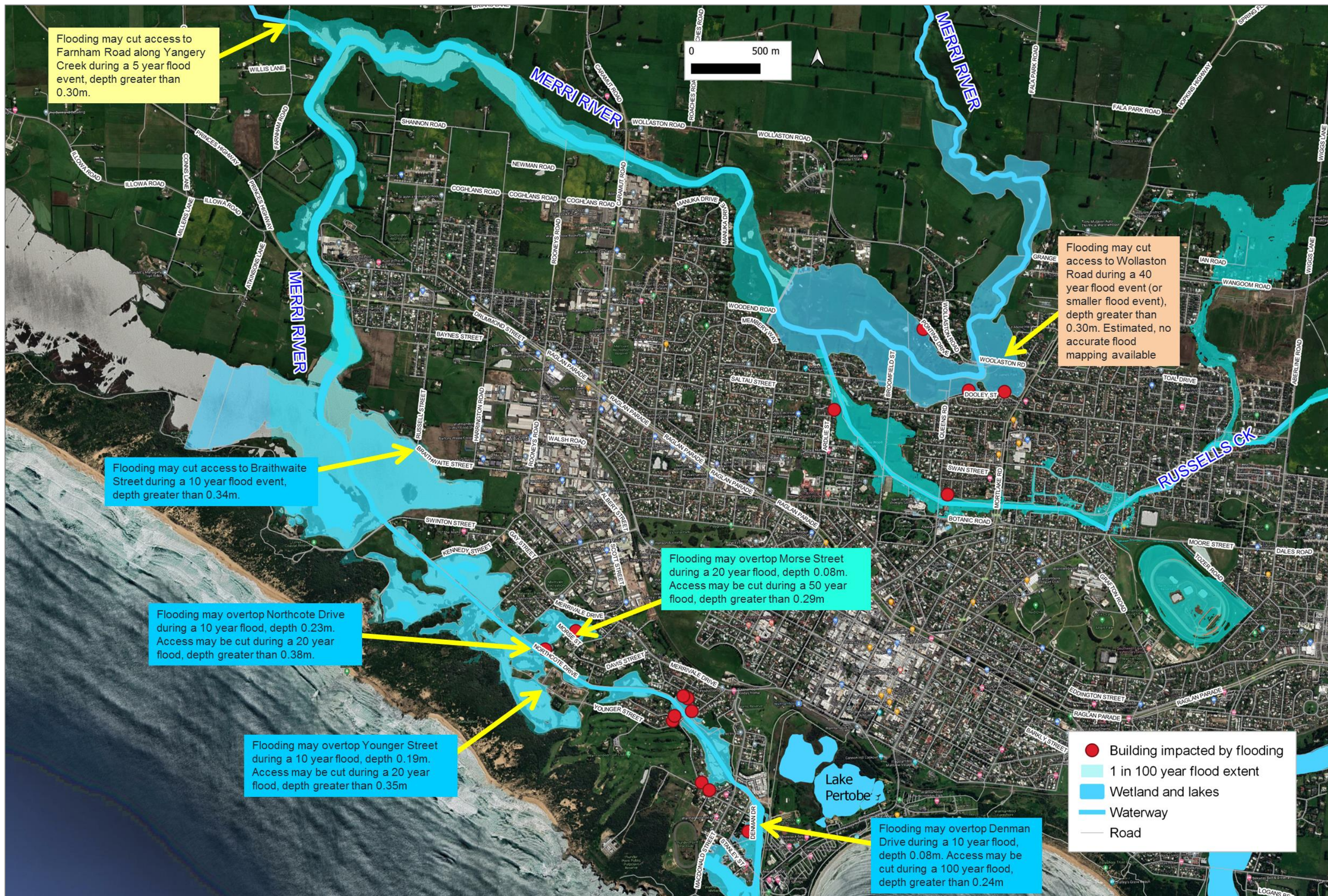
Figure 47. Warrnambool and Merri River catchment roads impacted by flooding for a range of design and historic flood events (Water Technology 2007).
