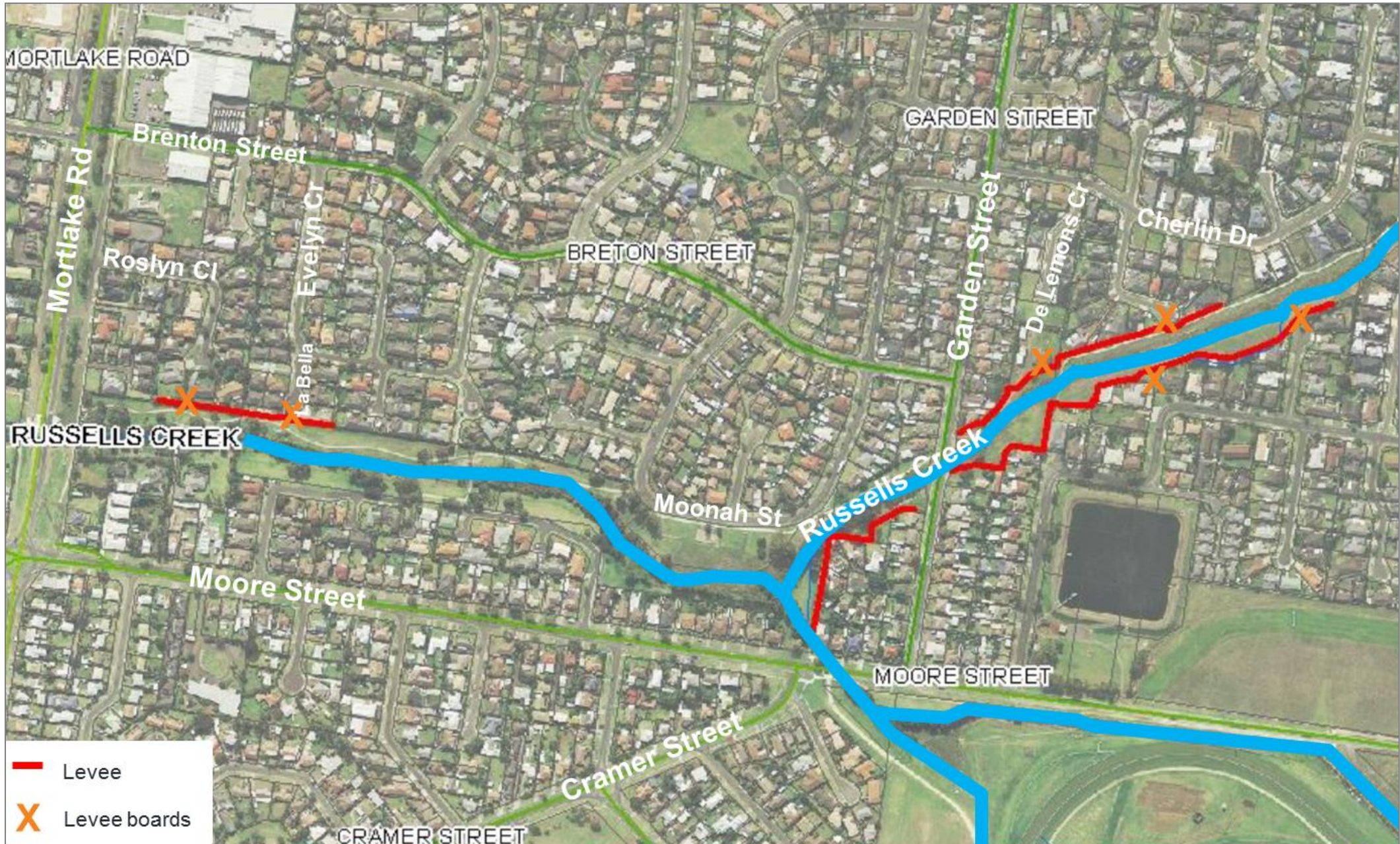
Figure 19. Russells Creek levee and board locations.
