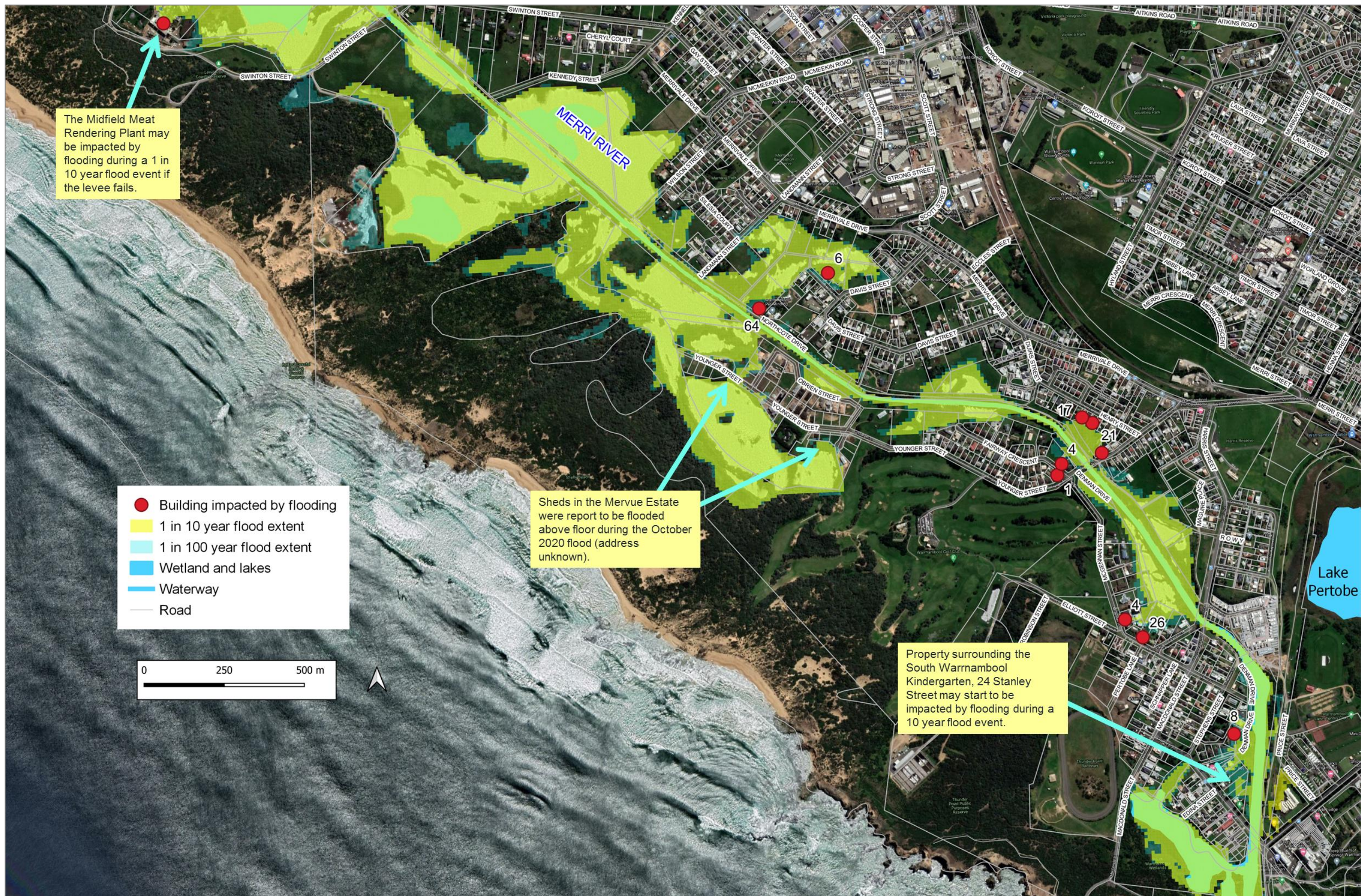
Figure 44. Buildings within the Merri River catchment impacted by flooding during October 2020 event (VICSES Request for Assistance Database).
