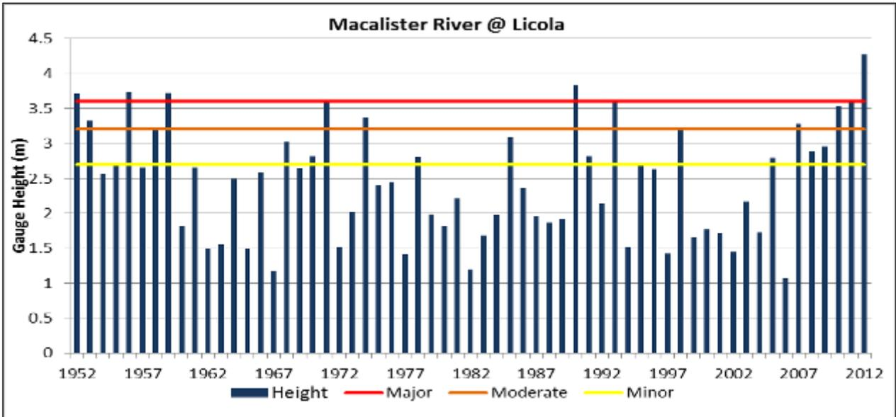
\* The gauge was washed away in 2007 and does not show the correct value
