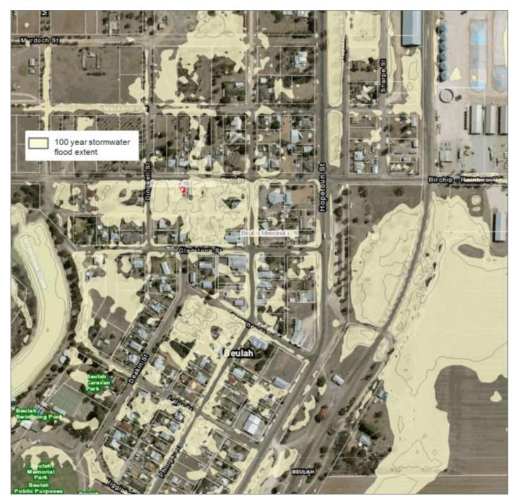
Beulah stormwater flood mapping, 100 year 2 hour duration (Water Technology 2006)
