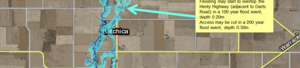
Roads impacted by flooding along the Yarriambiack Creek, north of Warracknabeal with the 200 year ARI flood extent.
