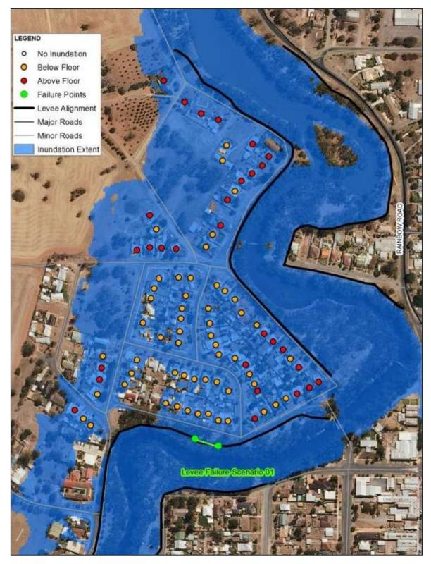
Impact assessment of the levee failure scenario.
