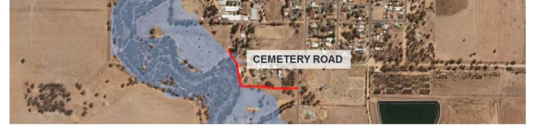
Roads and assets impacted by flooding in Warracknabeal, with the proposed levee and 100 year ARI extent (Water Technology 2016).
