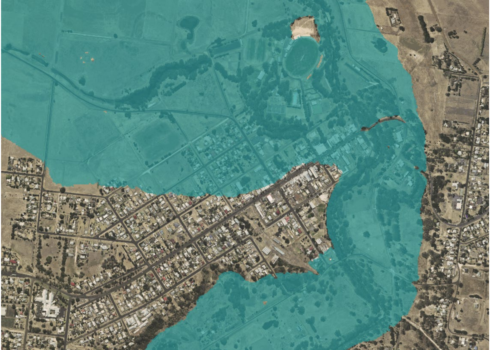
FloodZoom – Glenelg River @ Casterton, 1% AEP Extent (1 in 100 ARI) (Northern part of township)
