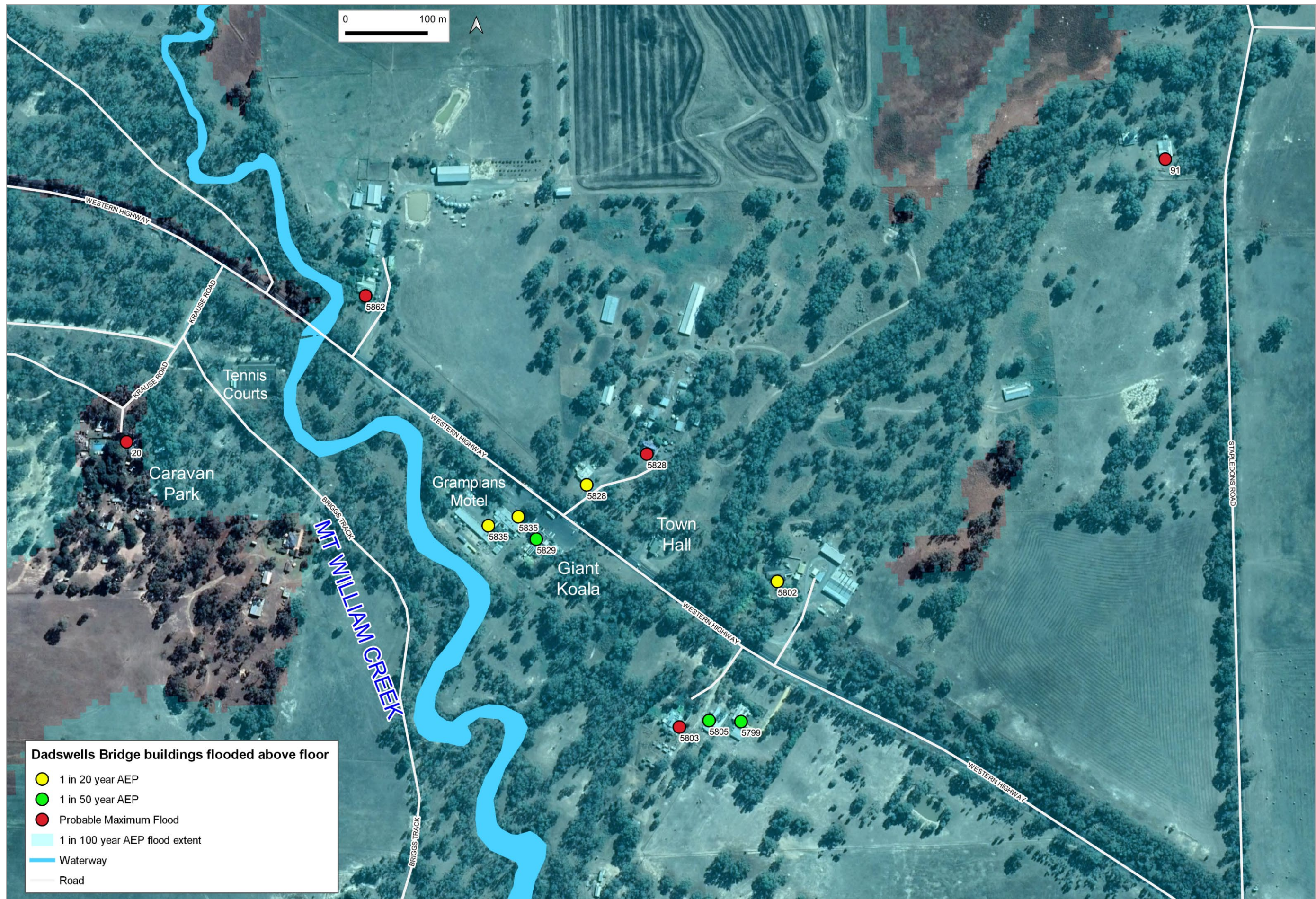
Figure 48. Dadswells Bridge buildings flooded above floor.
